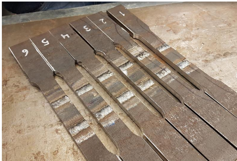
(c) The sides of the specimen are milled out.
