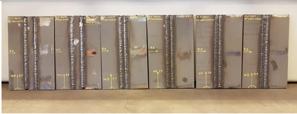
(h) All production plates ready to be forwarded for NDT and mechanical testing.
