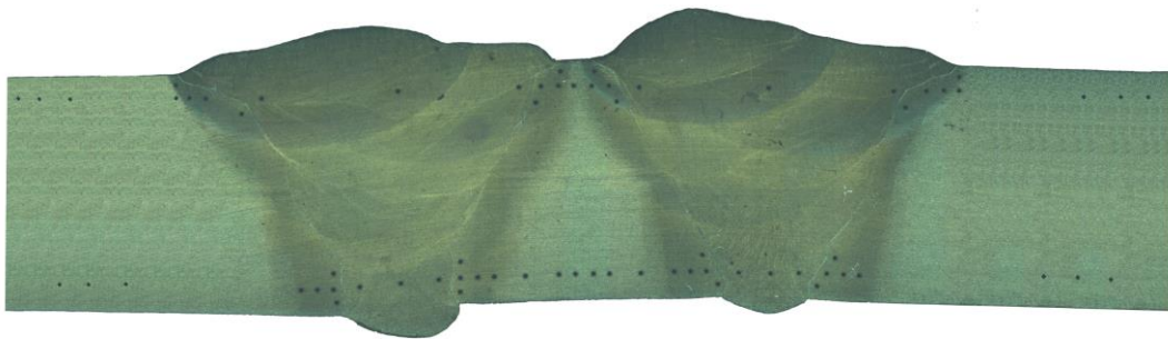
(c) Macro start – PL7 Weld A left, Weld B right.
