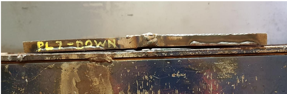
Figure 9-11 - Weld distortion after second weld PL7.
