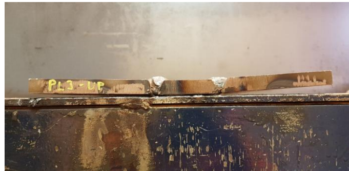
(e) Deformation after welding
