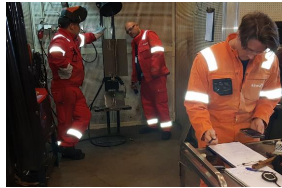
(h) Welding and Logging of qualification plate
