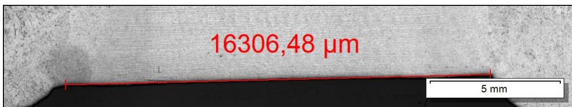
Figure 8-14 - Distance between weld toes was approximately 16 mm.
