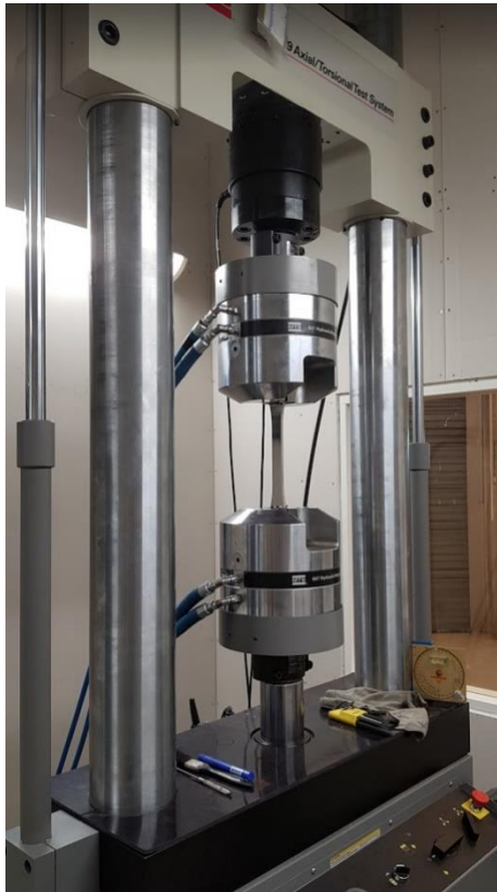
Figure 9-1 – MTS 809 Axial/Torsional Test System and dimensions. The lower grip is the actuator and the upper grip is static while testing, but can be manually moved by adjusting the overhead crossbeam.
