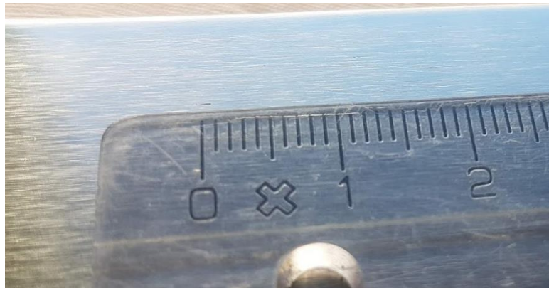
Figure 9-14 – Location of a small defect in the base material surface where fracture occurred.
