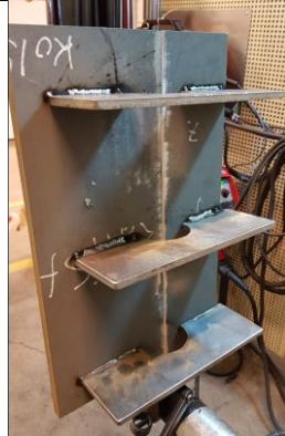
(b) Installation of strongbacks PL3.
