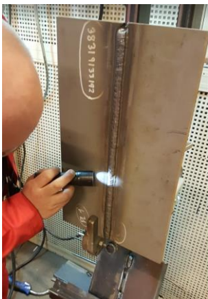
(i) Visual inspection
