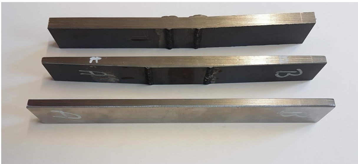
Figure 9-12 – Machining of fatigue specimens from welded S420G2+M plates in order to remove stress concentrations and misalignments the top face was initially machined until parallel followed by the machining of the bottom face.
