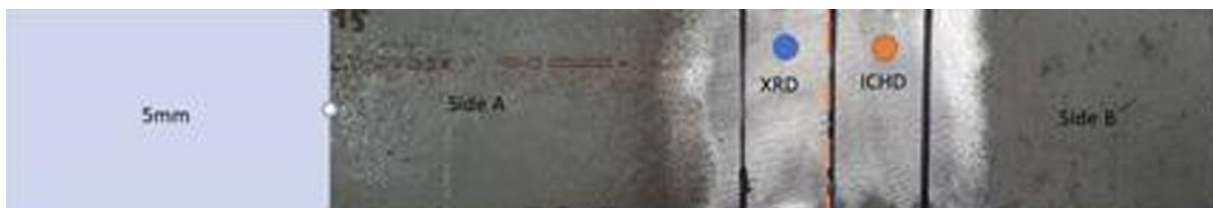
Figure 10-6 - Specimen test locations in the as-welded specimen.
