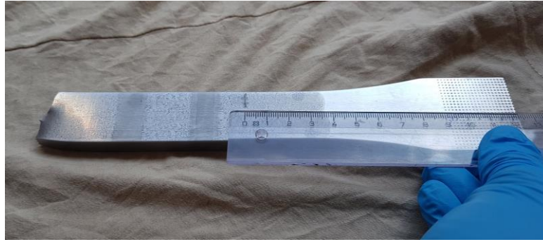
Figure 9-13 – Final fracture and location of crack initiation of 8612-3 A3 specimen.
