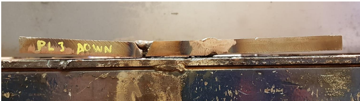
Figure 9-9 – Weld distortion after second weld PL3.
