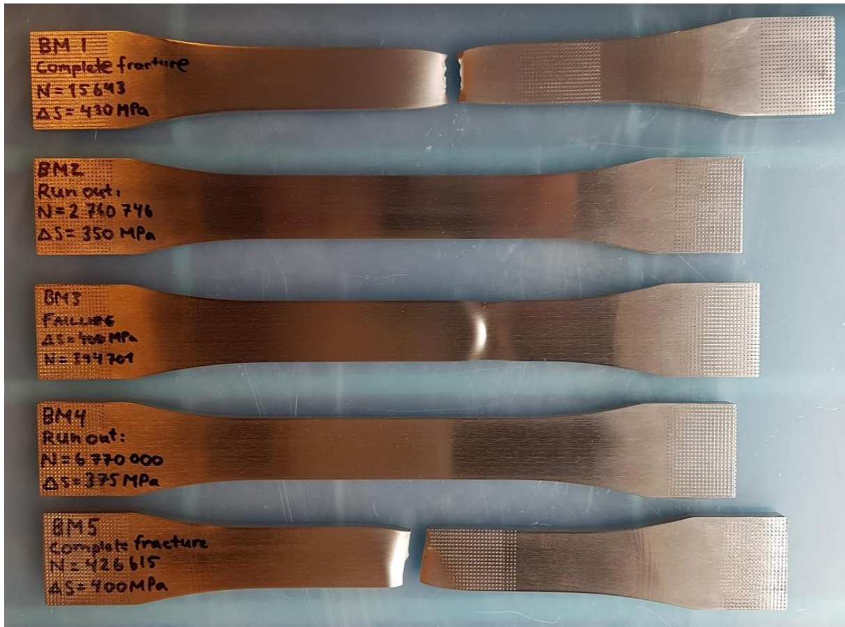
Figure 9-8 - Unwelded base material fatigue specimens after testing.
