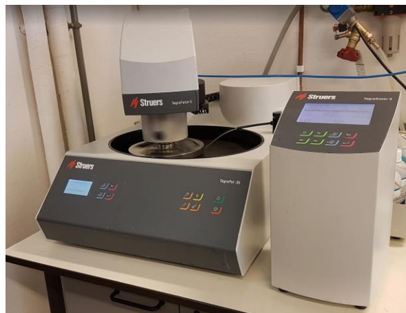
Figure 8-1 - Struers grinding and polishing machine including TegraForce-5, TegraPol-35 and TegraDoser-5.
