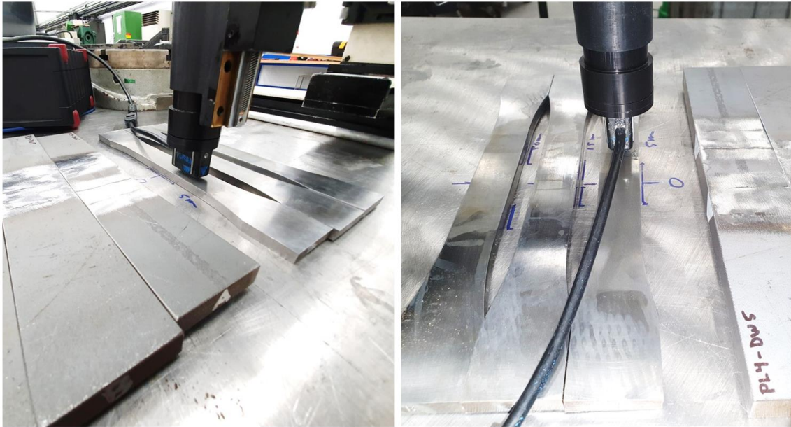
Figure 10-5 - Ultrasonic Residual Stress Measurement.
