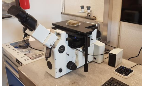
Figure 8-2 - Olympus GX53 Optical microscope.
