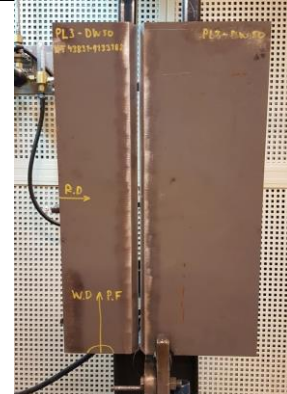
(c) PL3 fit-up preparation before welding of the first root in weld A.
