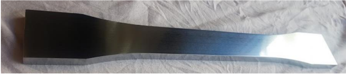
Figure 9-7 - Finished test specimen sample.
