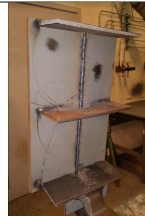
(f) Root pass of single-V groove weld, backside PL6.
