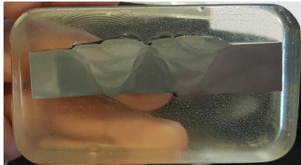
Figure 8-3 – Polished with 1 \mu\text{m} polishing cloth and subsequently etched with 2 % nital.
