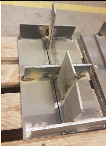
(f) Second strongbacks with extra middle support.
