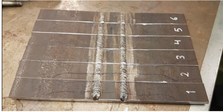
(a) The test plate was cut into 6 parts and each specimen received a ID. The plate thickness was 10mm. What is missing in the picture is the letter F (fatigue) on specimen F1-F5 and the letter T (Tensile) on specimen T6.
