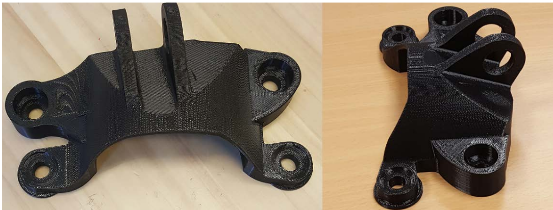
Figure 12. Additive manufactured final engine bracket design.
