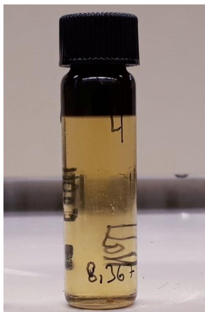
Figure 4.7 Effluent glass sampled during the hydrostatic loading phase, containing 1.5g oil
