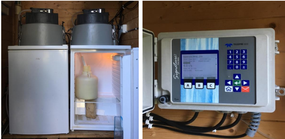
Figure 3-10 The ISCO 6712 Full-Size Portable samplers for inlet and outlet of Pond 2 connected to a container inside a refrigerator, placed inside the red sampling house. The picture to the right shows the flowmeter registering the flow data and transmitting pulses to the samplers. (13.05.19)
