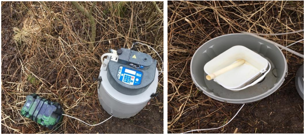
Figure 3-9 To the left: The automatic sampler connected to a car battery for power supply. To the right: The inside of the sampler showing the sample container during weekly water sampling. (06.02.19)
