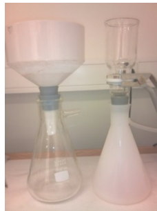
Figure 14. Vacuum filters with a Büchner funnel (Left) and a 47-mm funnel (Right)
