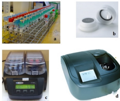
Figure 16. a) Dr. Lange cuvette test kits, b) Pall syringe filter holder, c) Dr. Lange thermostat LT 200, d) Dr. Lange spectrophotometer DR 5000
