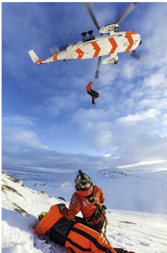
Figure 1. A search and rescue hoist rescue involving a Westland Sea King, with a rescuer on the ground with the patient. An anesthesiologist is in the hoist, which is operated by the flight engineer and system operator in the cargo door (photograph from training, courtesy of Norwegian Air Ambulance).
