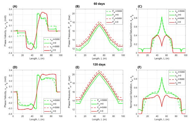
Fig. 9. Comparison for the horizontal compressible model for a WAG process with and without fluid-fluid interaction effects. The situation after 60 and 120 days are plotted. (A) Phase velocity at 60 days. (B) Phase pressure at 60 days. (C) Normalized saturation at 60 days. (D) Phase velocity at 120 days. (E) Phase pressure at 120 days. (F) Normalized saturation at 120 days.
