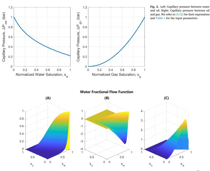
**Fig. 3.** Water fractional flow function  $f_{w}(s_w, s_o)$  (defined in (4.27)) with effects of model inclination  $\theta$  and total flow direction of  $U_T$ . (A):  $sin\theta = 0$ ,  $U_T = \overline{Q}_p/2$ ; (B):  $sin\theta = 1$ ,  $U_T = -\overline{Q}_p/2$ ; (C):  $sin\theta = 1$ ,  $U_T = \overline{Q}_p/2$ .
