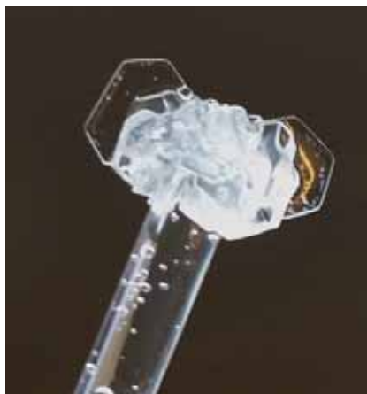
Figure 4. 10 THF hydrate crystals grown on the tip of the hollow glass tube.
