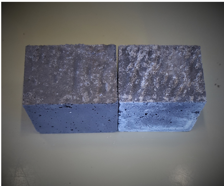
Carbonated cured in the left side Reference in the right side
