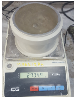
Figure 3.18: Density container filled with fresh cement paste
