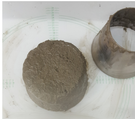
Figure 3.20: Slump test for cement mortar (W/C=0.3)
