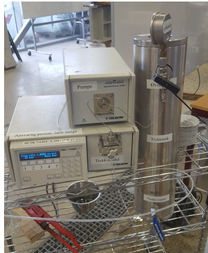
(b) Pressure tank (50 bar)
