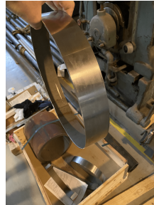
(b) The cladding alloy is separated from the backing steel.
