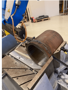
(a) The material is circularly cut by SCK 400 before lathing.
