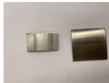
(c) The cladding alloy is machined carefully with Diskotom.
