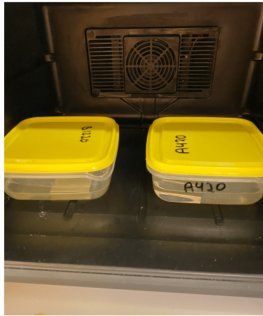
Figure 3.2: Picture of coupon experiment set up, where two coupons were contained in each container in three different refrigerators
