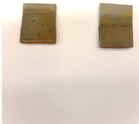
Figure 4.6: SS316L 2.5%Mo with weld in 4 degrees for 120 days, sides of the specimen shows heavy corrosion.
