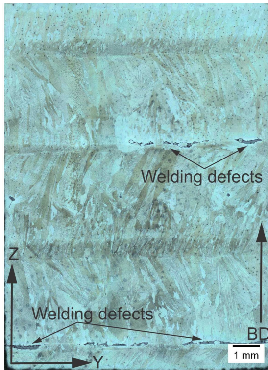
Figure 43: Welding defects of 30 min heat treated specimen, YZ-section
