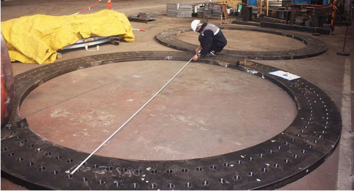
Figure 9 - Anchorage plate (Ciltug Inc., 2019)
