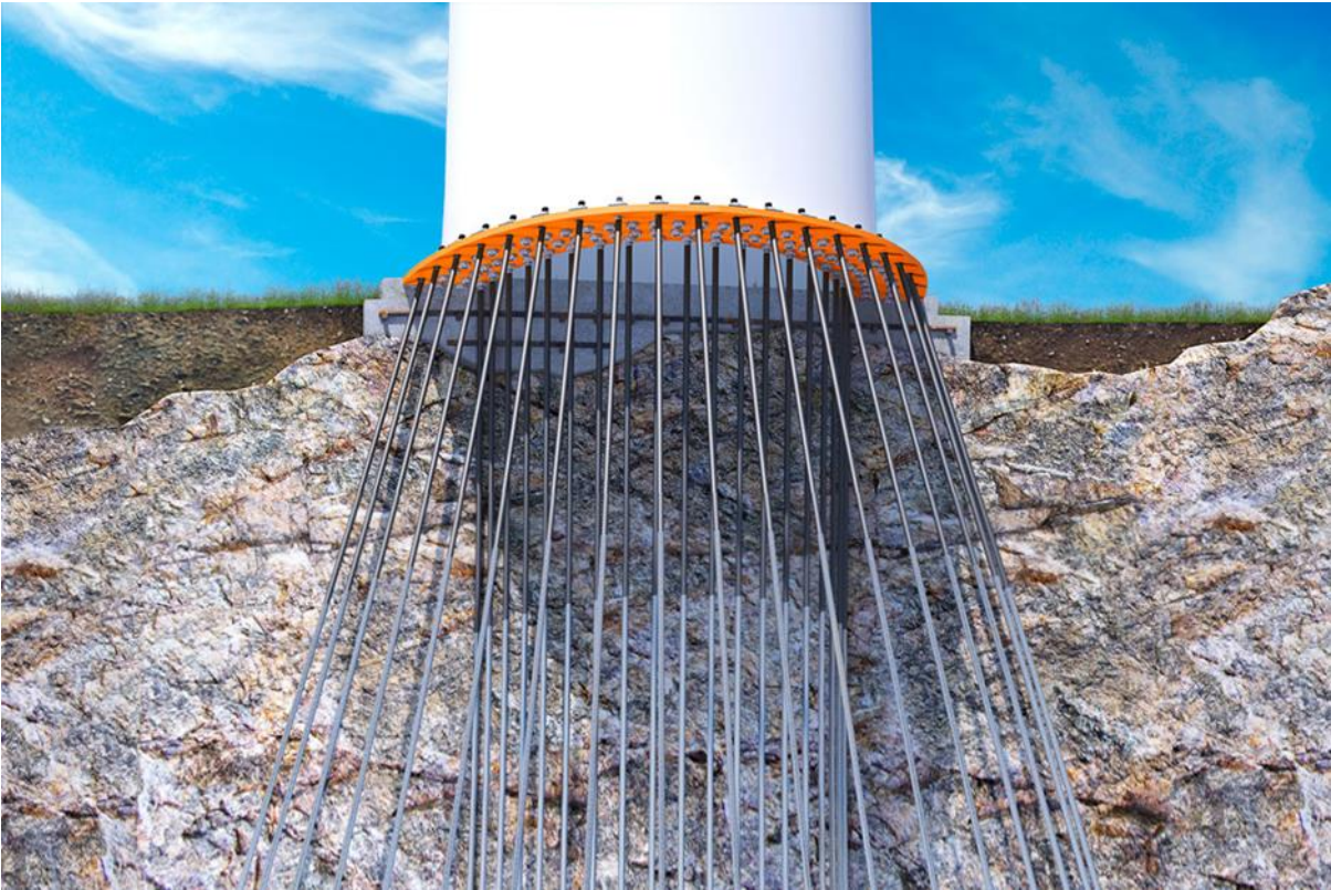
Figure 12 - Cross-sectional 3D view of a rock-piled foundation with an anchorage plate (Proplate, 2020)
