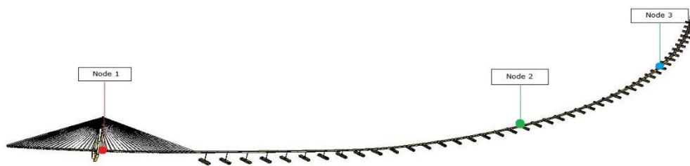
Figure 34 - Locations on the bridge for check of acceleration
