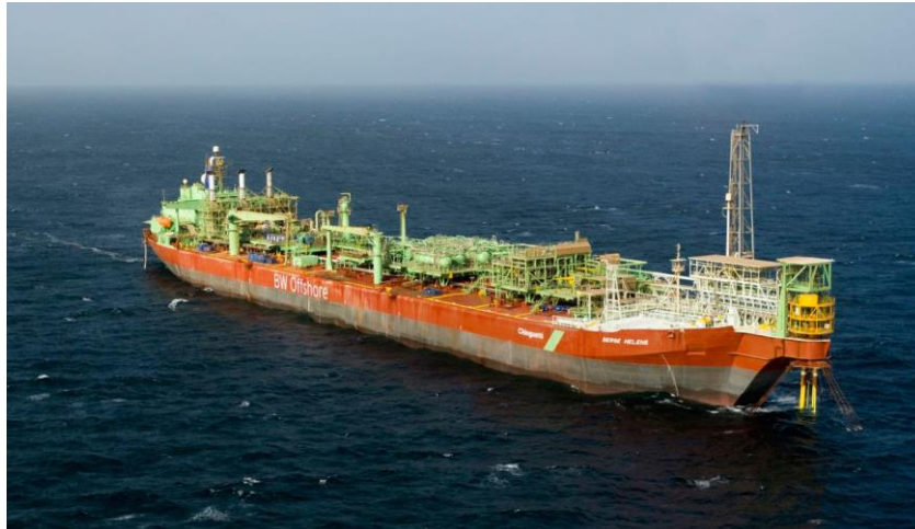
Figure 7 Berge Helene FPSO moored with permanent external turret solution.
