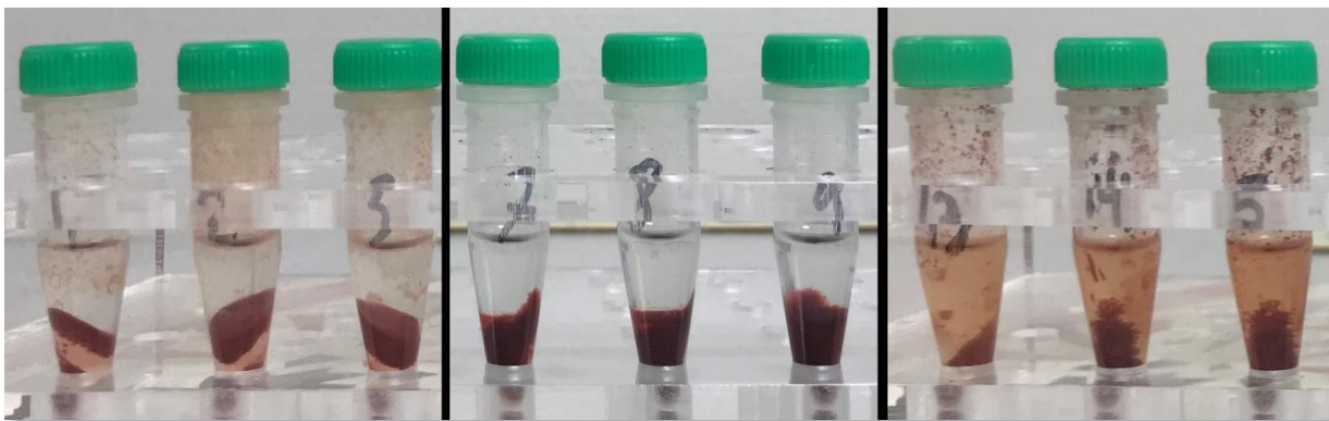
Figure 4-2 Three images demonstrating difference in phase separation. Samples were prepared with NaCl (5 M, 100 \mu L), MeOH (10 \mu L) and ACN (390 \mu L) (left image); NaCl (5 M, 100 \mu L), MeOH (50 \mu L) and ACN (350 \mu L) (middle image); NaCl (5 M, 100 \mu L), MeOH (100 \mu L) and ACN (200 \mu L) (right image).
