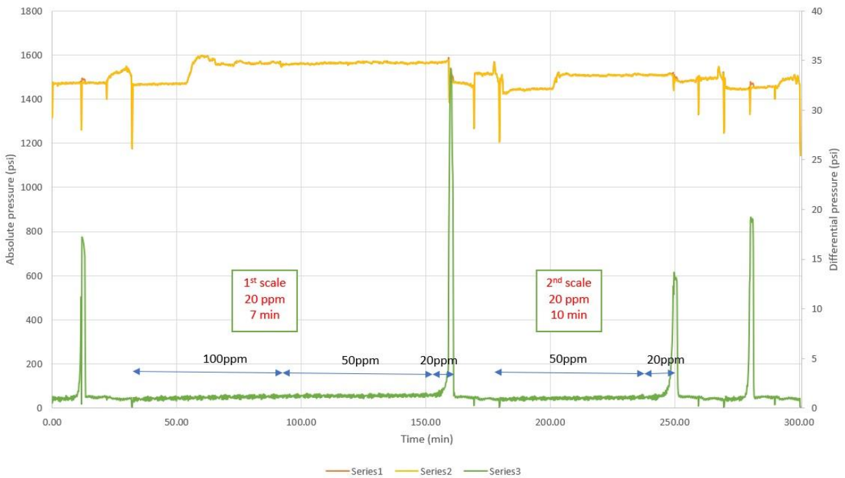
Figure 39. Failed inhibition concentrations of SI-8 for sulphate scale after thermal ageing.
