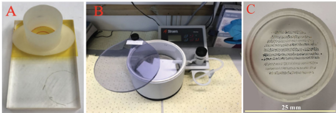
Figure 6: A) A FixiForm placed on the tape acts as a casing for the epoxy; B) The CitoVac machine used to apply vacuum and distribute the epoxy; C) How a finished unpolished heavy mineral mount looks like (sample MAG4). Scalebar is 25 mm.
