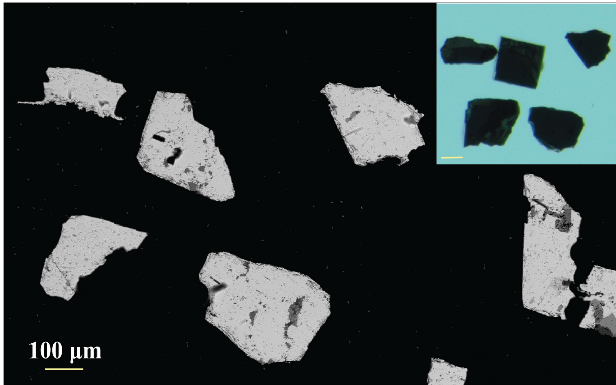
Figure 19: BSE image displaying pyrite grains in the Cancañiri sample. Inset image of the same pyrite grains, taken with an optical microscope (scalebar is 100 \mu\text{m} ).
