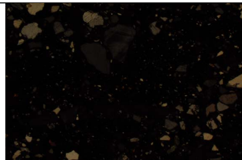
Fig. 6: As Fig 5, under crossed polarised light (XPL); note silt layer between sands.
