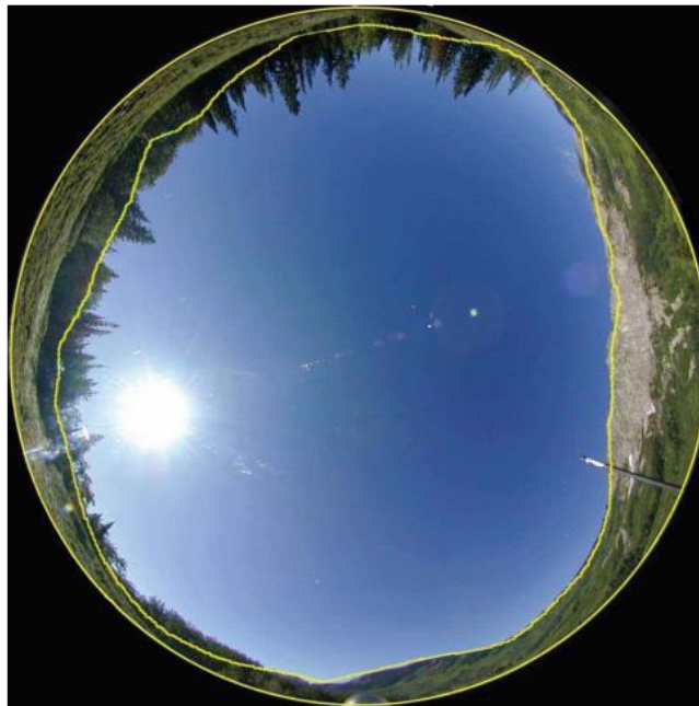
Figure 3-10- Hemispherical viewshed photo with calculated viewshed (yellow inner line). (Falklev, 2017)
