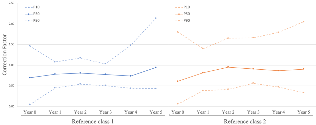
Figure 5.6: Side-by-side representation of the P90, P50 and P10 correction factors resulting from RC 1 and RC 2
