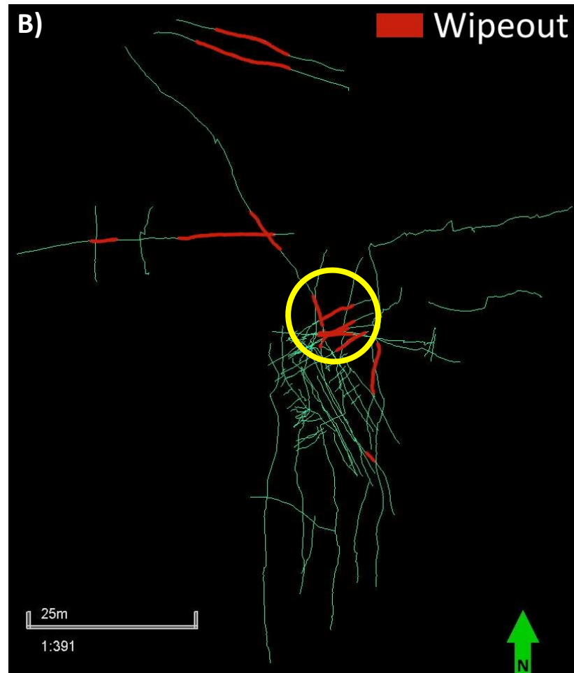
Figure 3.17: Locations of all wipeouts in A) the Upper Cemetery and B) the Middle Cemetery. It is possible to see that the same wipeout can be seen in multiple lines in some areas (circled).
