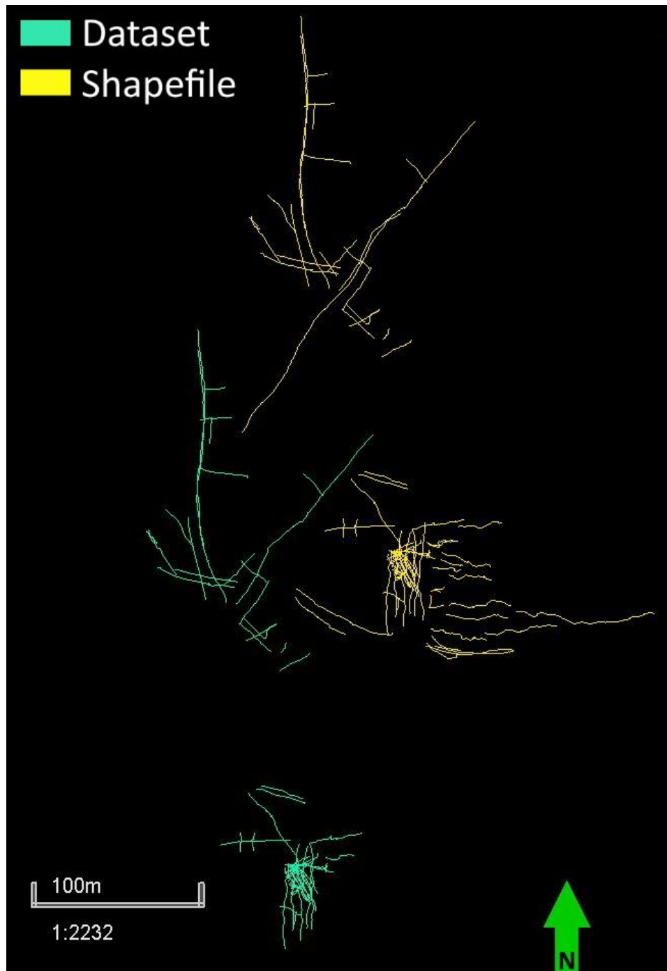
Figure 4.2: The interpreted dataset and shapefile displayed together in Petrel. It is clear that the interpreted dataset is shifted to the southwest, most likely due to a problem in the processing code.
