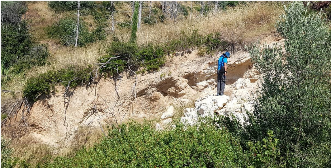
Figure 3.4: An outcrop of soft, white marl overlain by a harder calcareous sandstone. Photo taken at Station 24.
