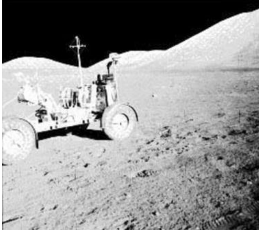
Figure 1.1: The surface electrical properties experiment carried out on Apollo 17 used a 3-component vector receiver mounted on the lunar rover on a dual axis multi-frequency dipolar antenna laid out on the surface (from Annan, 2002).
