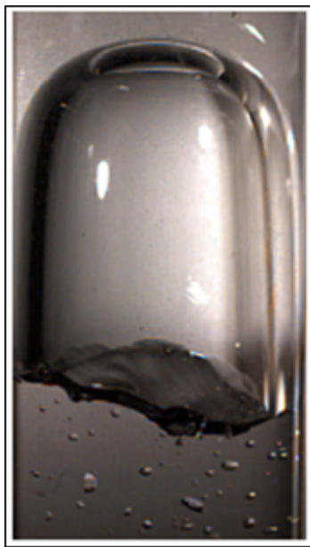
(a) Photograph of a Taylor Bubble moving upwards with no flow in pipe
