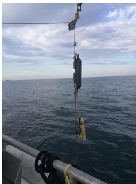
Figure 4 – Seawater sampling. A volume of 12 L seawater was collected near sea bottom from marine stations using a Niskin water sampler.
