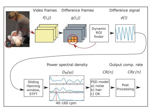
Figure 7.2: Simplified block scheme of the proposed system for chest compression rate measurement. Image frames from the smartphone front camera is used as input and output is the detected compression rate, CRf(n).
