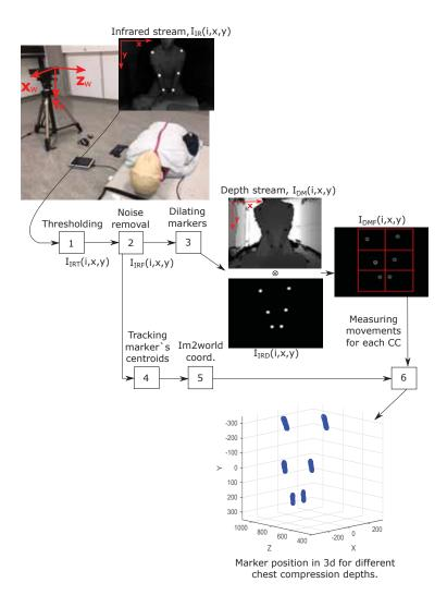
**Figure 9.1:** Block scheme of 3d CC modeling using Microsoft Kinect.  $I_{IR}(i, x, y)$  and  $I_{DM}(i, x, y)$  are provided by the Kinect.
