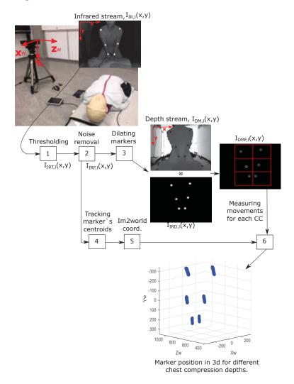
**Figure 3.11:** Block scheme of 3D chest compression modelling using Microsoft Kinect.  $I_{IR,l}(x, y)$  and  $I_{DM,l}(x, y)$  are frames provided by the Kinect camera.
