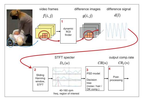
Figure 3.3: Simplified block scheme of measurement of chest compression rate. Input: image frames from the smartphone camera. Output: the detected comp. rate,  $CR_f(n)$ .
