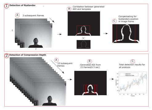
Figure 3.8: Proposed system for detection of compression depth. Top: detecting bystander and regions of interest (ROIs). Bottom: detection of compression depth.
