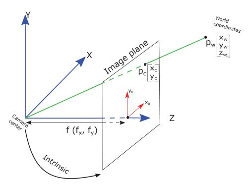
**Figure 2.1:** A model of the connection between the camera center, image plane and world coordinates.  $f_x$  and  $f_y$  is the focal length of the camera,  $x_0$  and  $y_0$  the principal point offset from the image center,  $p_w$  a point in the real world and  $p_c$  the point in the image plane.
