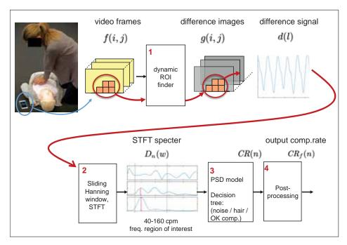
**Figure 6.1:** Simplified block scheme of QCPR cam-app 2.0. Input: image frames from the smartphone camera. Output: the detected comp. rate,  $CR_f(n)$ .
