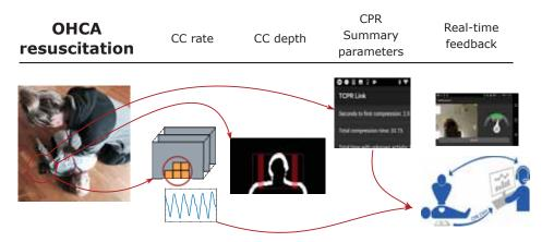
Figure 1.2: An overview of the proposed system for automatic video analysis in outof-hospital cardiac arrest situations. Video frames from the smartphone camera are utilized in algorithms for measurement of chest compression rate, chest compression depth and CPR summary parameters, and the *real-time feedback* section illustrates how the feedback can be received by the bystander through a smartphone application and on a webserver for the dispatcher at the emergency unit.
