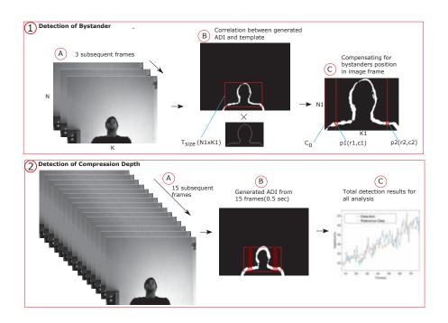
Figure 8.1: Proposed system for detection of compression depth. Top: detecting bystander and regions of interest (ROIs). Bottom: detection of compression depth.
