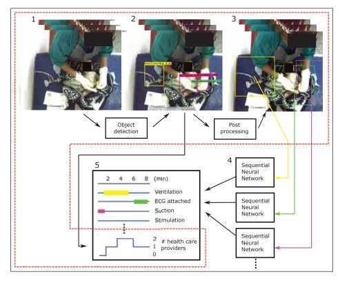
Figure 10.1: Block scheme of the activity detection system. The red dotted line encircles the steps proposed in this paper. 1: Generated dataset is input to YOLOv3 object detection network. 2: Detected objects. 3: Detected object area after post processing. 4: Sequence of images from areas are used as input to sequential neural networks. 5: Activity time lines is the final output.
