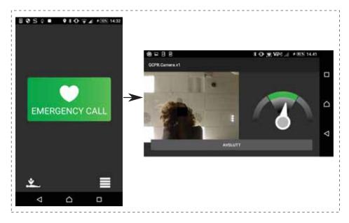
Figure 3.14: Smartphone app for establishing the emergency call and for bystander feedback during CPR.
