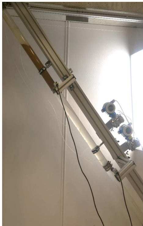
Fig. 4. 30 - Successful isolation by the laponite-based pill on 40° test setup
