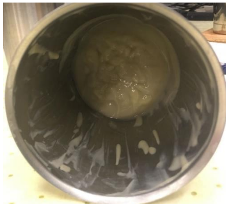
Fig. A. 2 - Bentonite pill of recipe 2.B in sample cup tilted to horizontal
