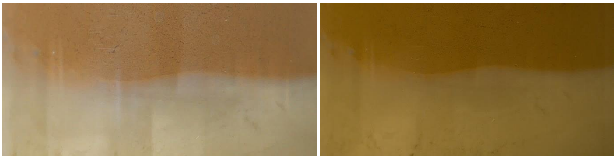
Fig. 4. 3 – Interface right after placement (left) and interface at end of test (right) on the vertical setup
