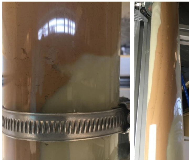
Fig. 4. 42 – Source of channel (left) and channelling of WBDF along the pipe wall (right)
