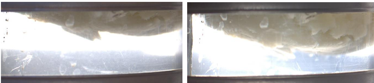
Fig. 4. 2 – Interface right after placement (left) and interface at end of test (right) on vertical setup
