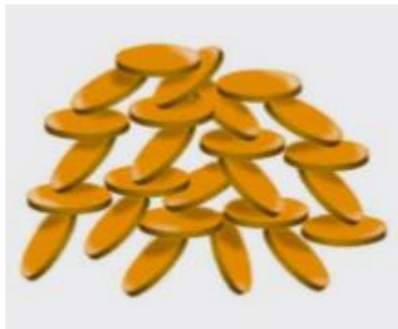
Fig. 2. 10 - House of Cards structure from gel formation (from BYK Additives & Instruments (2014))
