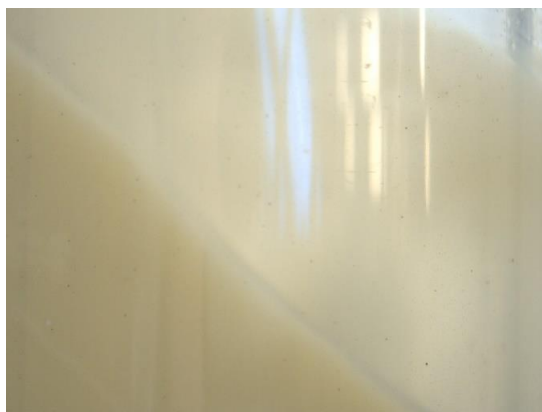
Fig. 4. 10 - Bentonite pill surface after placement with thin pill layer across the pipe wall
