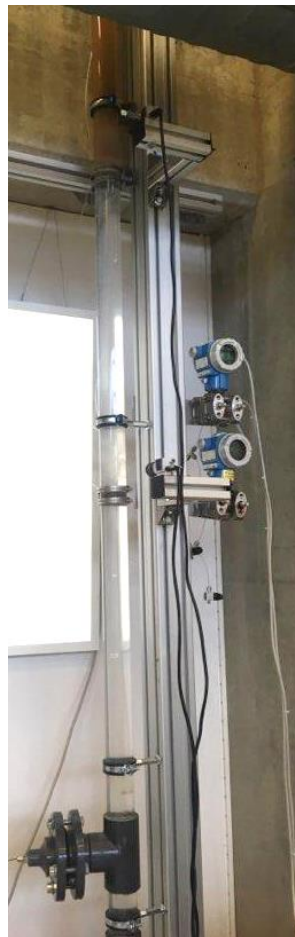
Fig. 4. 24 - Successful isolation by the laponite-based pill on the vertical test setup
