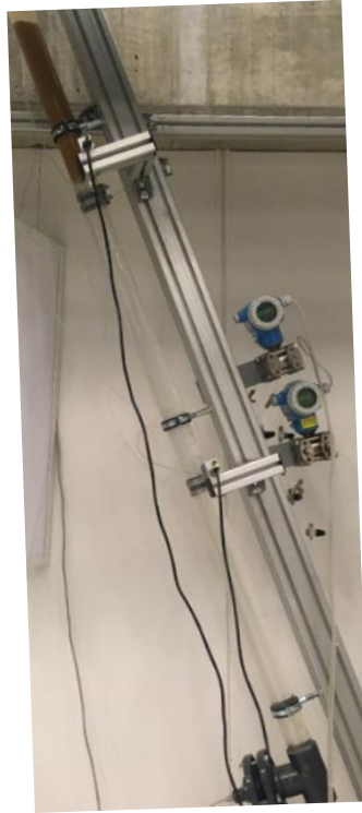
Fig. 4. 27 - Successful isolation by the laponite-based pill on 20° test setup
