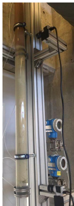
Fig. 4. 4 - Successful isolation by the bentonite-based pill on the vertical test setup
