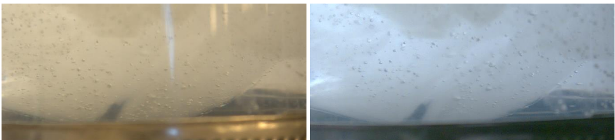
Fig. 4. 28 – Interface right after placement (left) and interface at test end (right) on the 40° inclined setup
