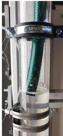
Fig. A. 7 – Foam removal using a hose
