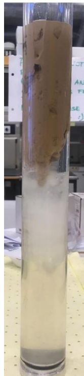
Fig. B. 9 – Channelling of WBDF through recipe 2.L
