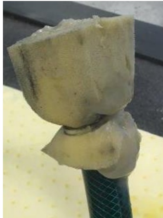
Fig. A. 8 - Pig used to clean the pipe wall and compress the pill from above
