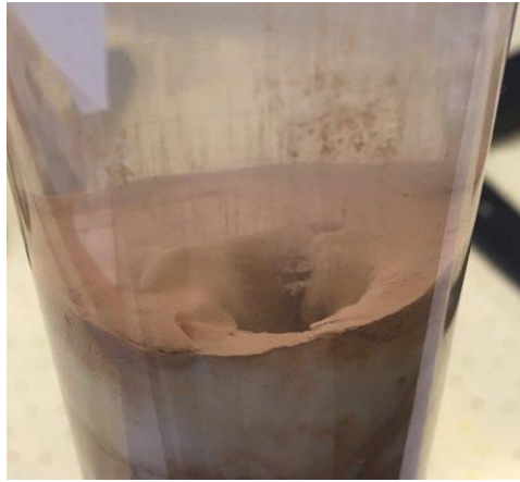
Fig. B. 7 - Source of WBDF channel created by pouring
