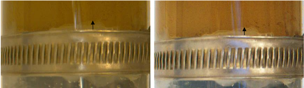
Fig. 4. 29 – Interface right after placement (left) and interface at test end (right) on the 40° inclined setup
