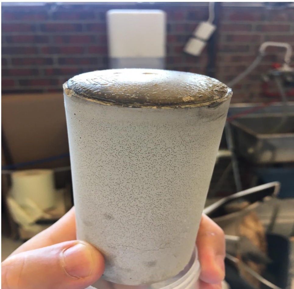
Figure 6-9 The Consequences of Gas Bubbles on Curing
