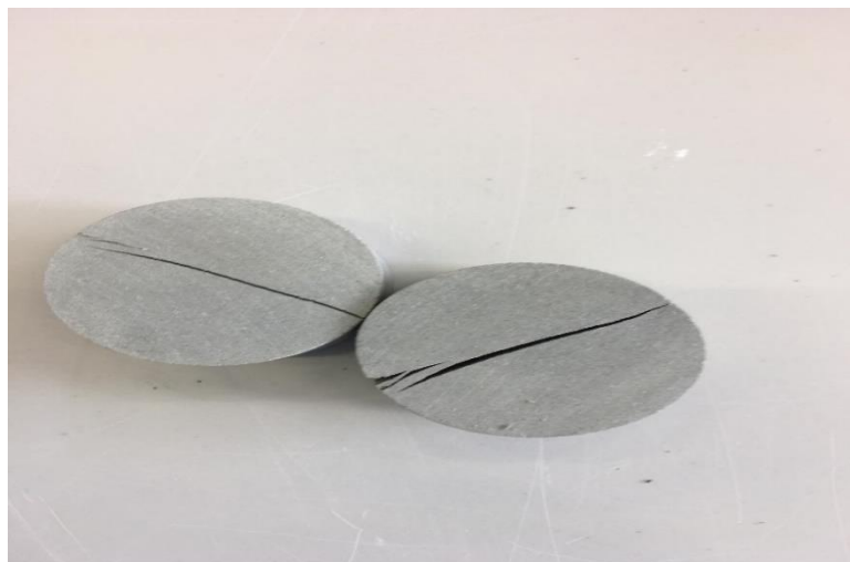
Figure 5-12 The crushed Sample from Indirect Tensile strength test
