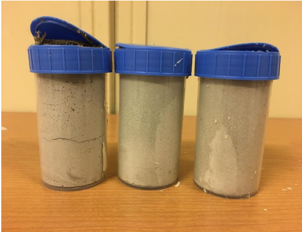
Figure 6-8 The Result of curing condition (under Atm Pressure)
