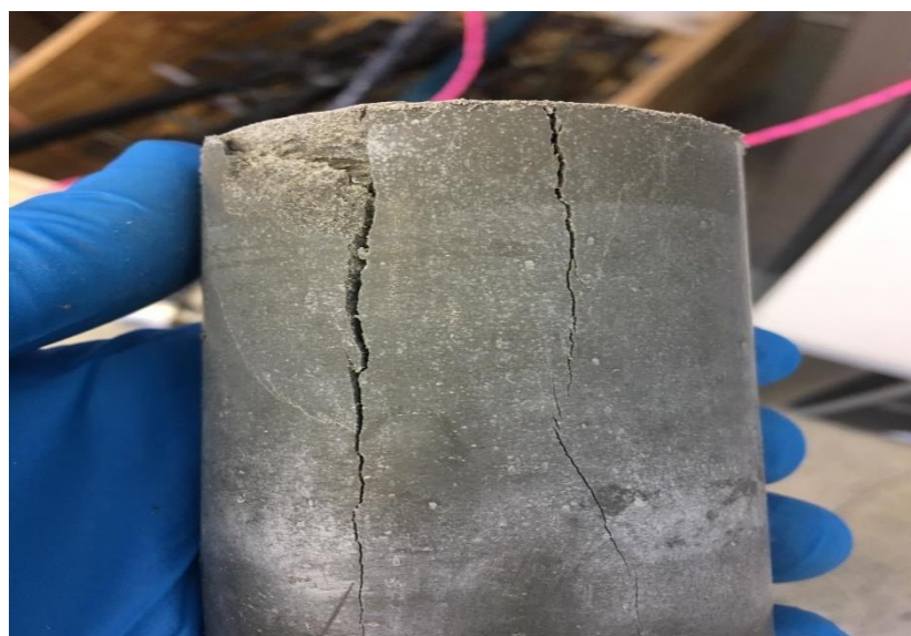
Figure 5-10 The Crushed Sample from uniaxial compressive strength test
