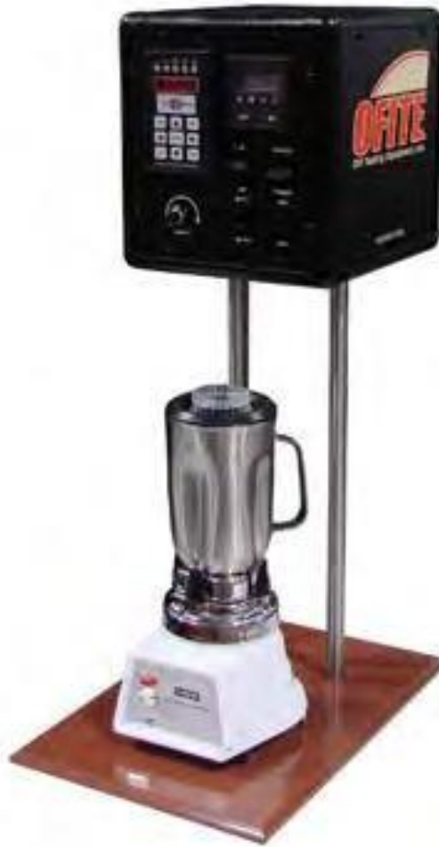
Figure 5-2 OFITE Model Commercial Blender
