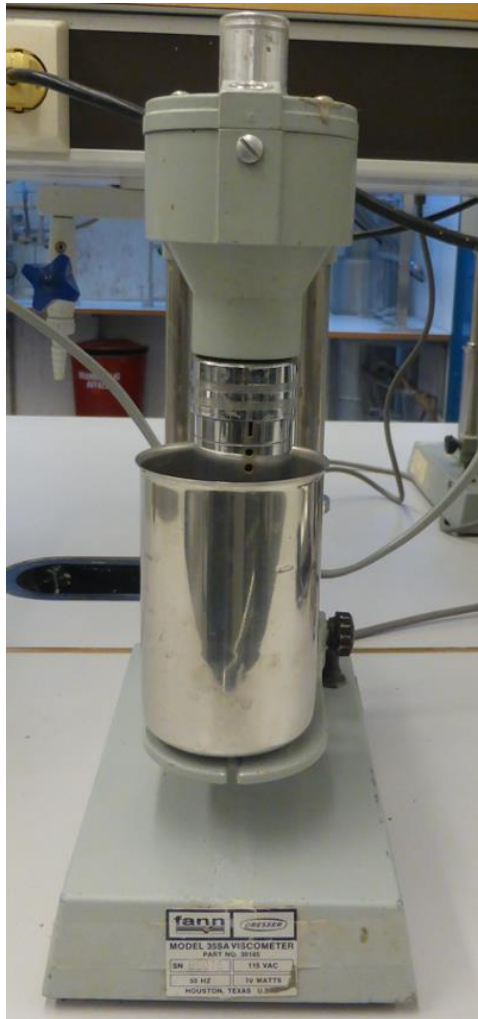
Figure 3.17 Fann 35 viscometer used for measuring rheology
