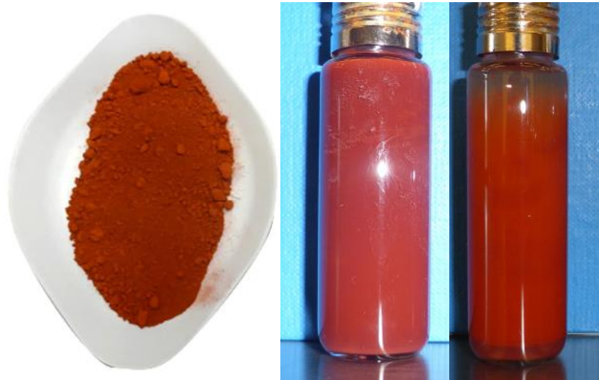
Figure 3.4 Iron oxide powder (left) mixture after mixing (middle) mixture after 48 hours (right)
