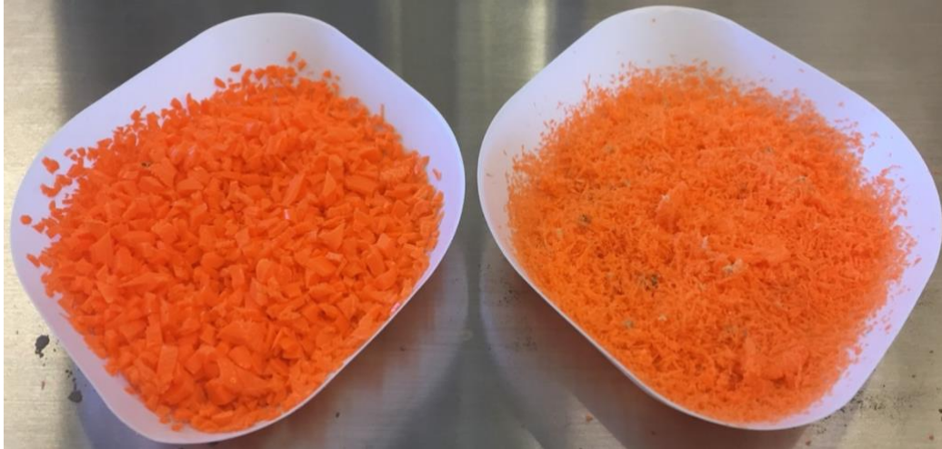
Figure 3.6 Silicone rubber coarsely cut (left) and finely cut (right)
