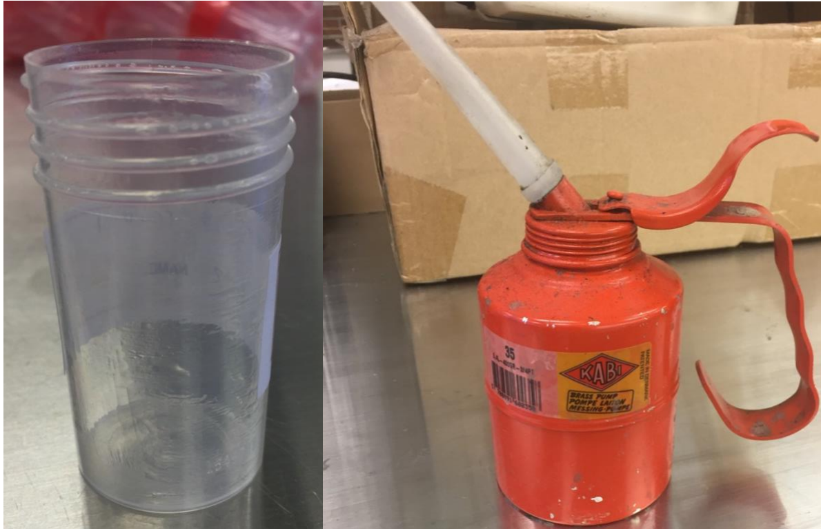
Figure 3.7 Cement mold coated in oil (left) and oil for lubrication (right)
