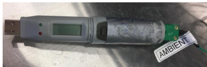
Figure 3.12 Temperature logger from ESK-EL
