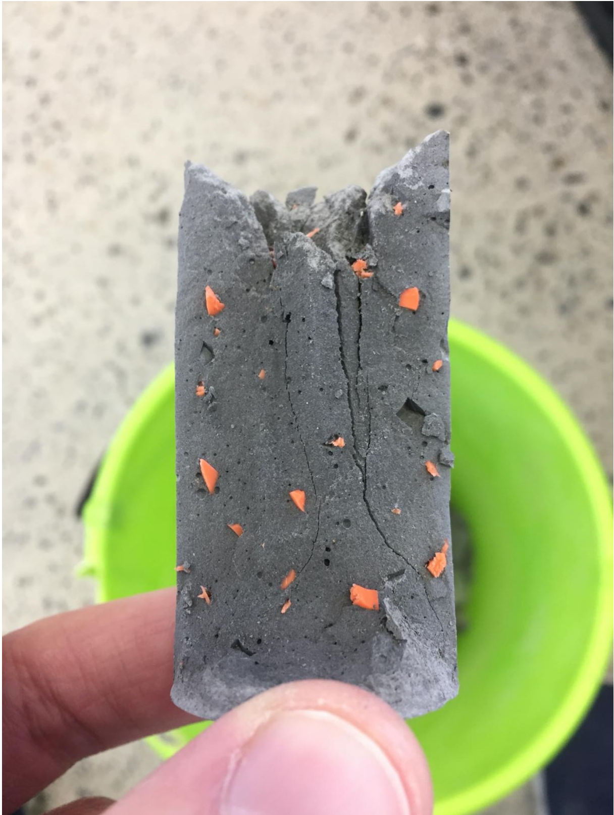
Picture above shows the inner structure of a sample containing rubber silicone after it was subjected to destructive testing. One can clearly see the difference in the finely and coarsely cut rubber.
