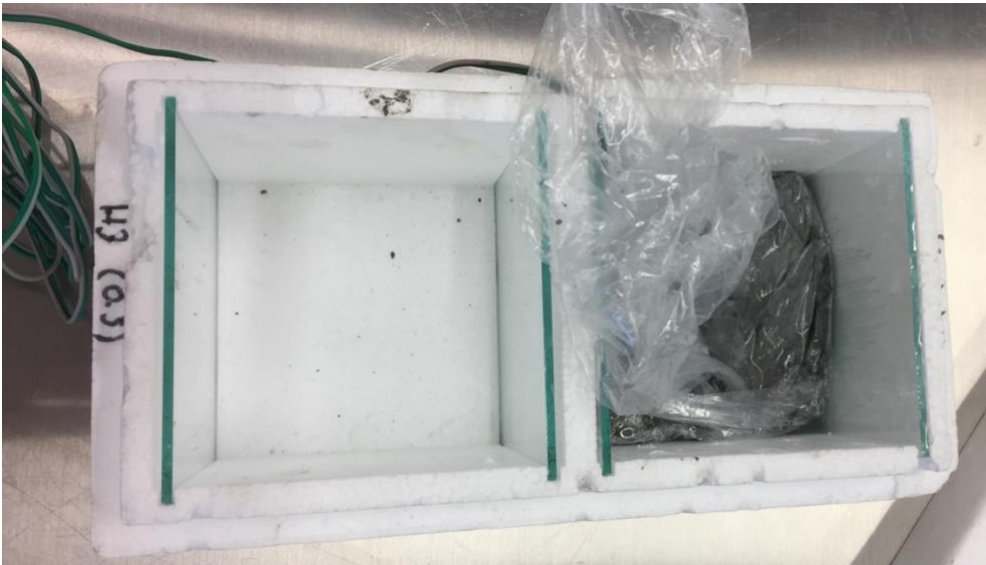
Figure 3.13 Styrofoam box used for temperature logging with cement in one compartment
