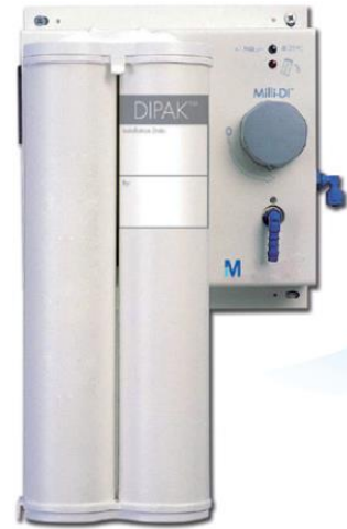
Figure 18 Merck Milli-DI 22 µM filter. Feedwater conductivity = 0.04 S/m and 0 ppm dissolved CO 2 . DI water quality resistivity > 1MΩ.cm at 25 °C. (Merck 2012)
