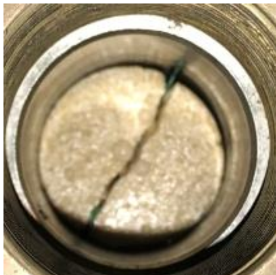
Figure 28 For mod SI tests spacers were placed between the two fractured halves allowing brine to contact the three open faces of each core half. The use of spacers also prevented the buildup of a pressure differential across the core that could force brine into the core.
