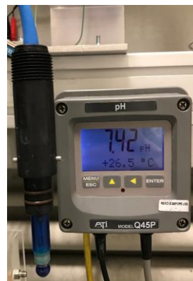
Figure 19 ATI model Q45 pH meter and sensor used to measure injection brine and effluent pH.
