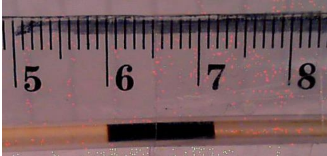
Figure 29 Volumetric measurements of oil were made by multiplying the length of an oil segment by the ratio of the inside tubing volume to its length. This was necessary because oil became trapped in the dead volume of the BPR during mod SI experiments of aged cores.
