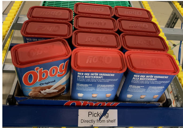
Figure 4.5: The figure displays the setup of the experiment. One product was skewed while the rest was in the original position. Because the skewed product occupies a larger area, the row in the back was removed. The other products were turned backward to force product detection to detect the skewed product.
