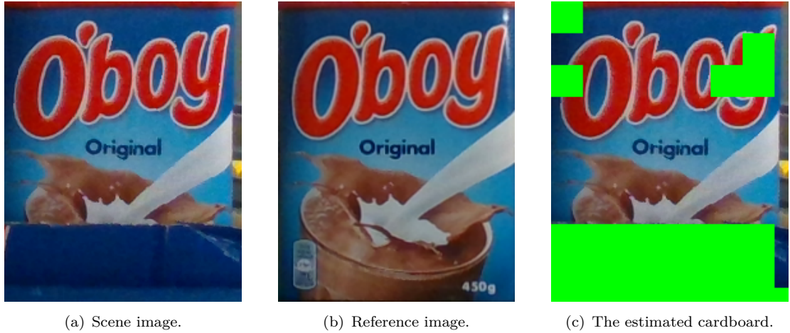
Figure 3.7: The figure illustrates the cardboard estimation on the product O'boy. Figure (a) is the scene image, with a perspective transform to align with the reference image (b). The result after conducting the evaluation is displayed in (c).
