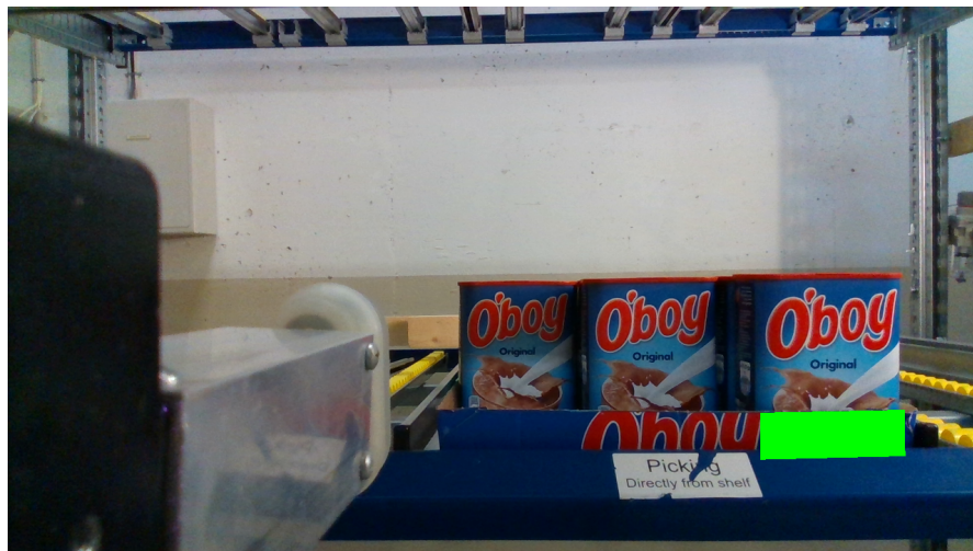
Figure 3.10: The figure displays the resulting cardboard estimation in front of the product, marked in green. As seen from the figure, the cardboard is only estimated in front of the detected product. With the estimated cardboard, this image is the basis for generating the collision map in section 3.4.
