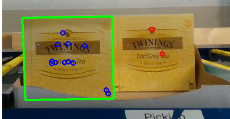
Figure 3.11: The figure shows the product of interest, marked with the green bounding box. The blue circles are the keypoint inliers, and the red circles are the keypoint outliers. This figure is cropped to only show information of interest.
