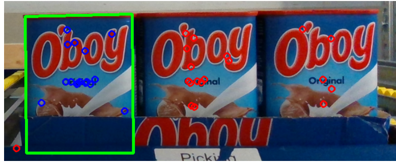
Figure 4.3: The image illustrates the product detection of the product "oboy01." The green bounding box is the estimated region of the product. The blue and red circles are not relevant to the image.
