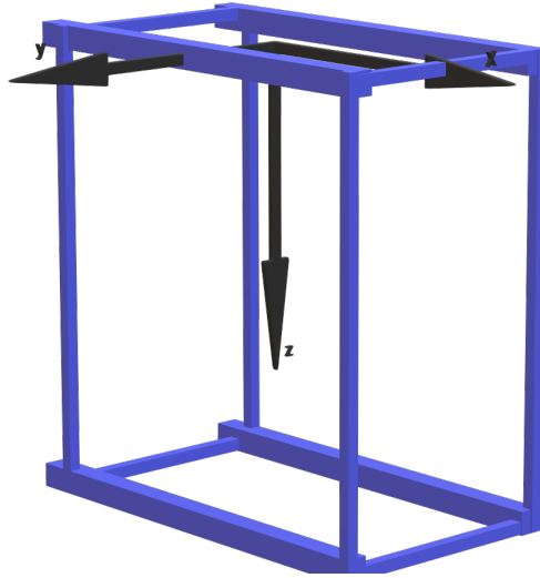
Figure 26: Depicting the drilling rigs global frame.
