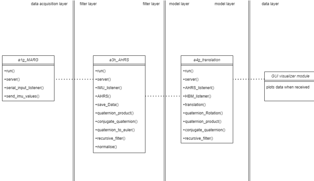
Figure 38: Class diagram for the Software developed for tracing the drill bit position. Dotted line indicates communication beyond the layers. Double lines indicate layer boundary.
