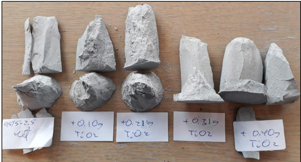
Figure Apx.6: A few pieces of the geopolymer reference #3 + TiO 2 plugs after UCS test, showing that internal visible pores exist.
