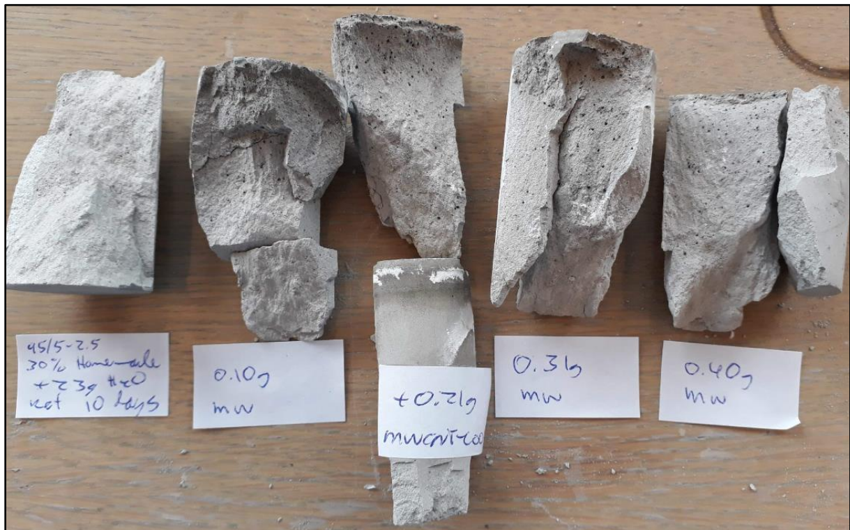
Figure Apx.4: A few pieces of the geopolymer reference #2 + MWCNT-COOH plugs after UCS test, showing that internal visible pores exist.
