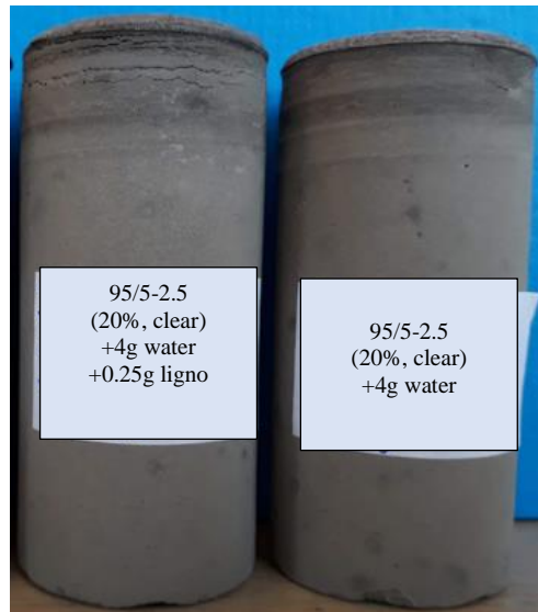
Figure 5.27: Geopolymer plugs cured 7 days in oven and exposed to ambient air in 48 days, TM#12.
