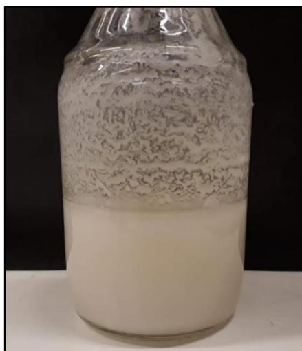
Figure 4.10: Homemade sodium metasilicate liquid (45.1%, milky color) at 40°C.
