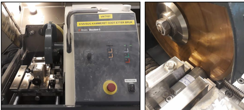
Figure 4.16: Struers Discotom-5 machine used to cut free water of the geopolymer plugs.
