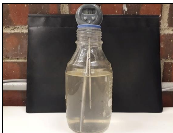
Figure 4.14: The homemade sodium metasilicate liquid (37.1%, clear) cooled down to 51.3°C.
