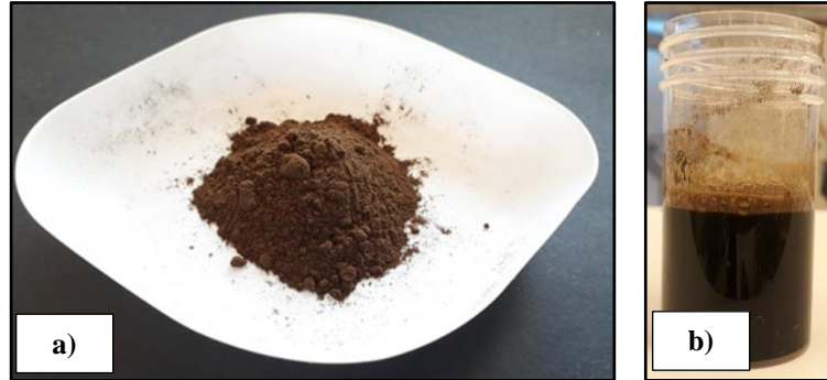
Figure 4.6: a) Lignosulfonate in powder state. b) 0.75g lignosulfonate dispersed in 23g water.
