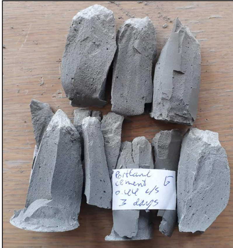
Figure Apx.1: A few pieces of the Portland cement plugs after UCS test, showing that internal visible pores exist.
