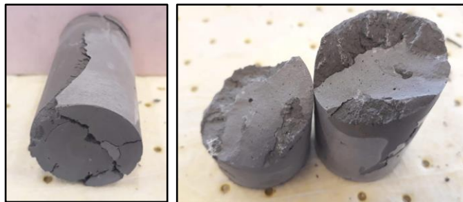
Figure 5.41: Portland cement cured in plastic cup without lubrication oil on inner surface.
