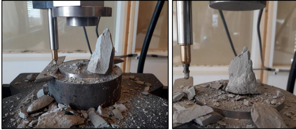
Figure 5.60: Two examples of (45.1%, clear) homemade-based geopolymer explosion when crushed.
