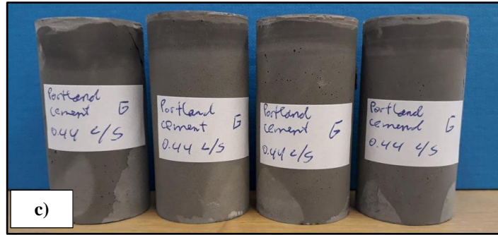
Figure 5.19: TM#8. a) plugs out of oven, side view. b) plugs out of oven, top view. c) plugs polished.
