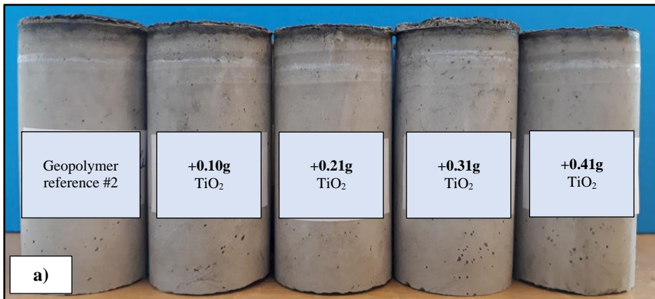
Figure 5.46: 3 days cured, TM#20. a) showing free water of the plugs. b) plugs cut to ~61mm, below free water interface
