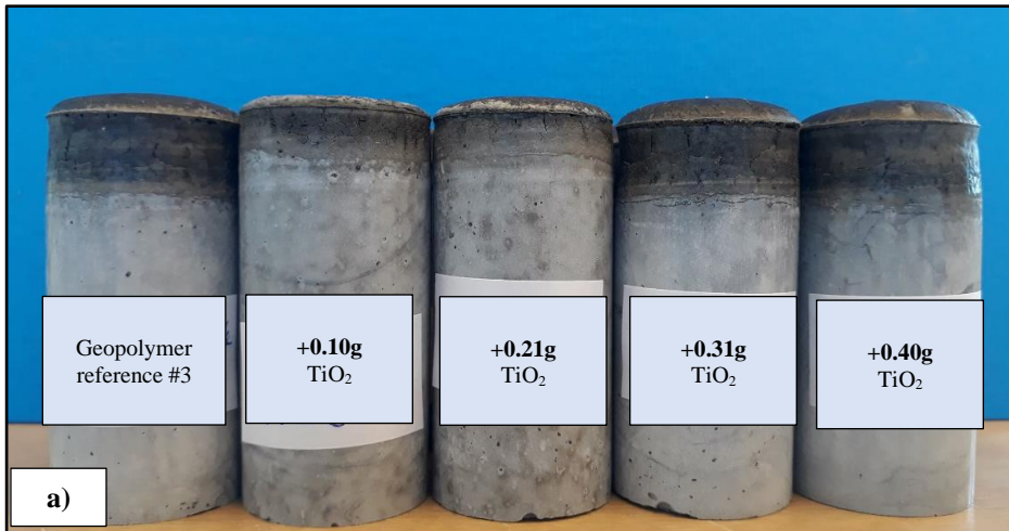
Figure 5.54: 3 days cured, TM#22. a) showing free water of the plugs. b) plugs cut to ~58mm, below free water interface.
