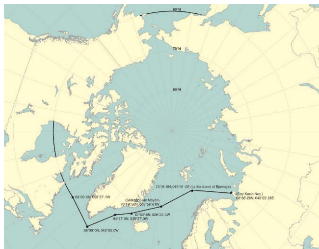
Figure 1. Maximum geographical extent of the Polar Code's area of application in the Arctic. The figure extracted from the Polar Code is for illustrative purposes only. For exact coordinates, the regulation refers to SOLAS Chapter XIV/1.3 [11].
