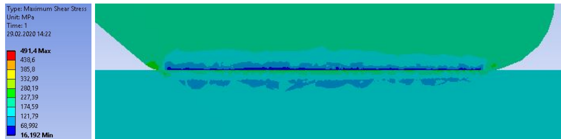
Figure 5.16: Cross-sectional view of 'section 1' for case 2 with axial force and 149°C.
