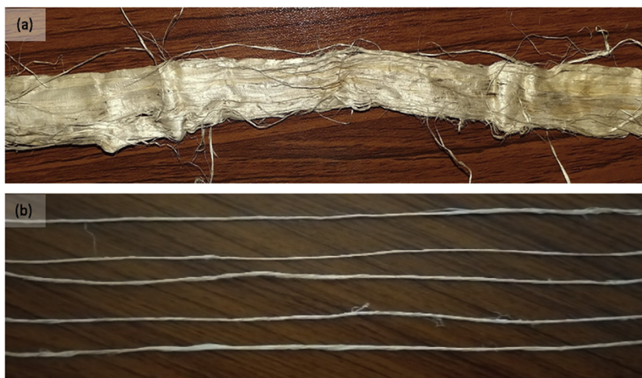
Fig. 2. Acacia fiber (a) Acacia tortilis raw fiber, (b) handmade acacia tortilis fiber yarn).
