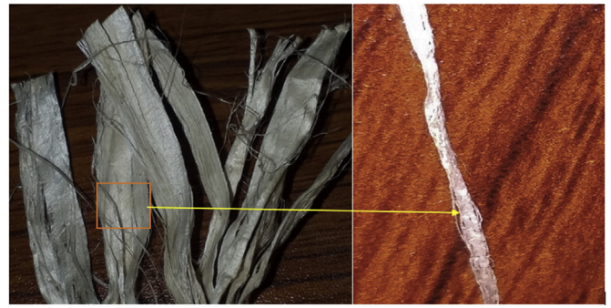
Fig. 3. Geometry of Acacia tortilis fibers (a) Acacia fiber appearance, (b) magnified appearance.
