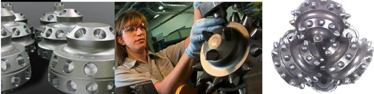
Figure 6.11: Showing the production of a tungsten carbide insert bit. From left: The holes are drilled in the cone, thereafter the inserts are pressed into the holes. The bit is then mounted to a final product. [4]
