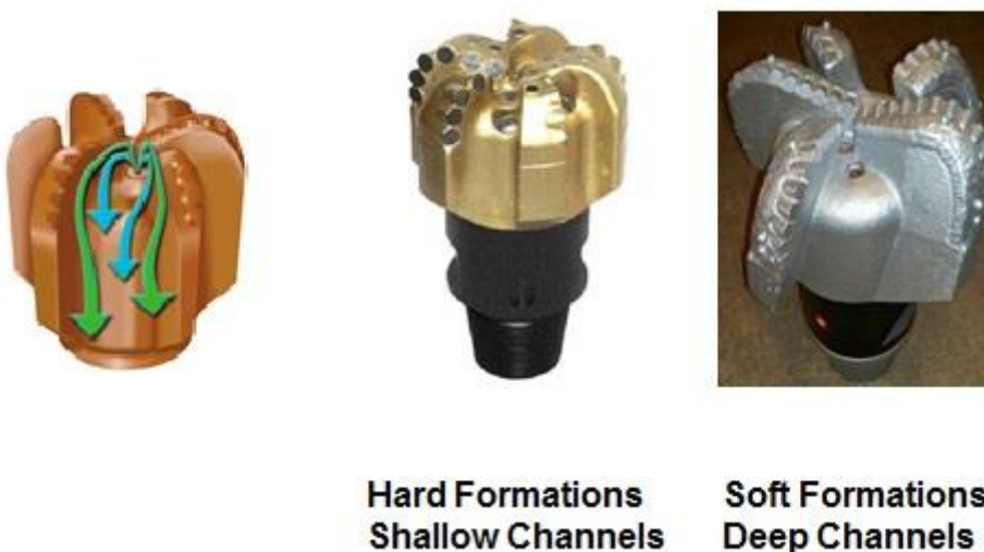
Figure 6.27: From left: The junk slot area of a PCD bit, a PDC bit with shallow channels used for drilling hard formations and a PDC bit with deep channels (large junk slot area) used to drill soft formations. [46]
