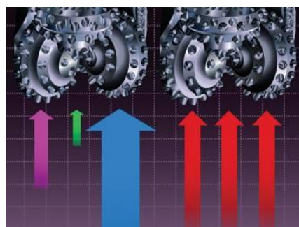
Figure 6.5: At left the roller cone is imbalance, and the cones bear more load than others. By using the balance technology, balance is achieved among all the cones. [7]
