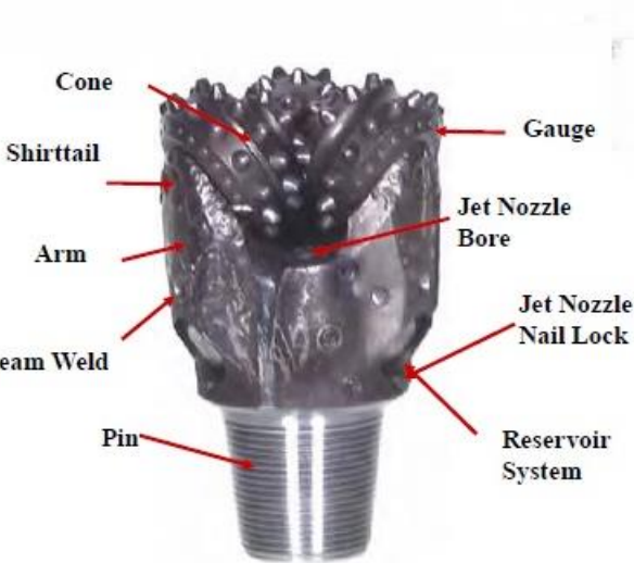
Figure 6.9: Shows the components of a roller cone bit. [4]
