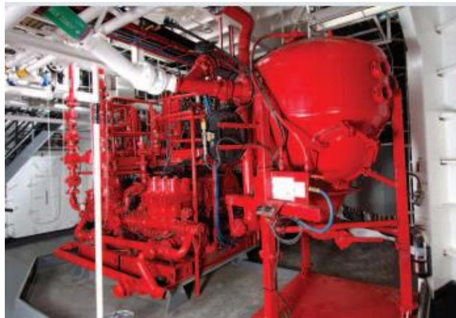
Figure 4.3: Halliburton cementing unit, the unit provides mixing, pumping and environmental performance. [32]
