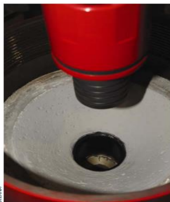
Figure 4.10: Shows a sealing sleeve adapter with Stab-In Float collar. [39]
