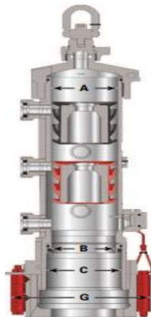
Figure 4.4: Halliburton high-pressure cementing head. 3 valves are available on this head. A bottom (red) and top plug (black) is pre-installed. [30]
