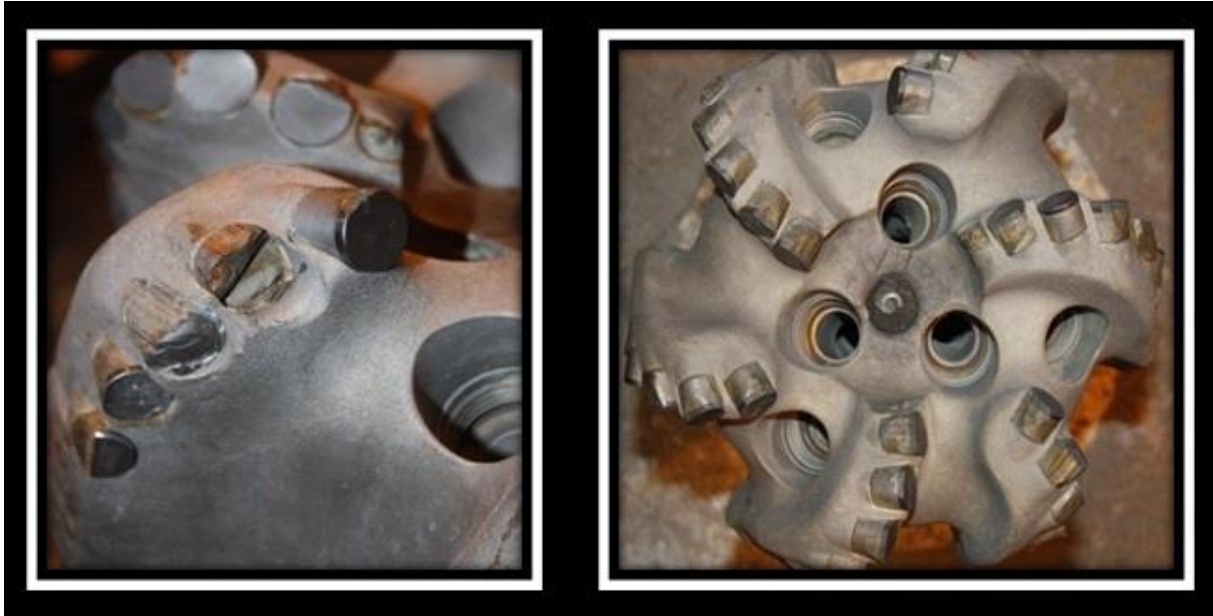
Figure 7.1: A worn PDC bit after drilling through shoetrack equipment. The picture shows broken cutters and large wear in the middle of the PDC bit. This bit drilled through some shoetrack equipment, then hitting the formation. The bit was then pulled out of the hole due to very low rate of penetration. [49]
