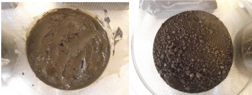
Figure 9. From the left, untreated and treated drilling waste.
