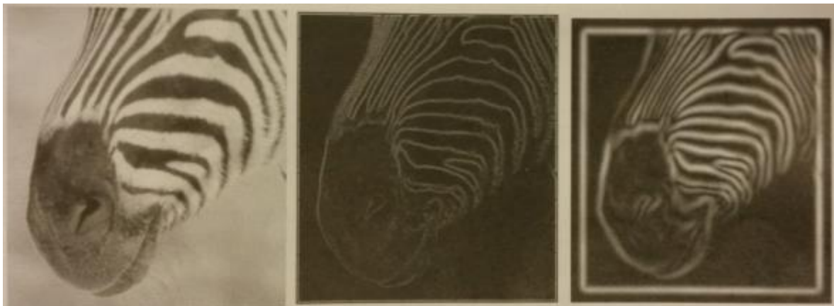
Figure 2-2. The gradient magnitude can be estimated by smoothing an image and then differentiating it. The smoothing will affect the gradient magnitude as seen above. At the center the gradient magnitude is estimated with a Gaussian smoothing scale of \sigma = 1 pixel. On the Right the gradient magnitude is estimated with a smoothing scale of \sigma = 2 pixel (Forsynth and Ponce, 2012).
