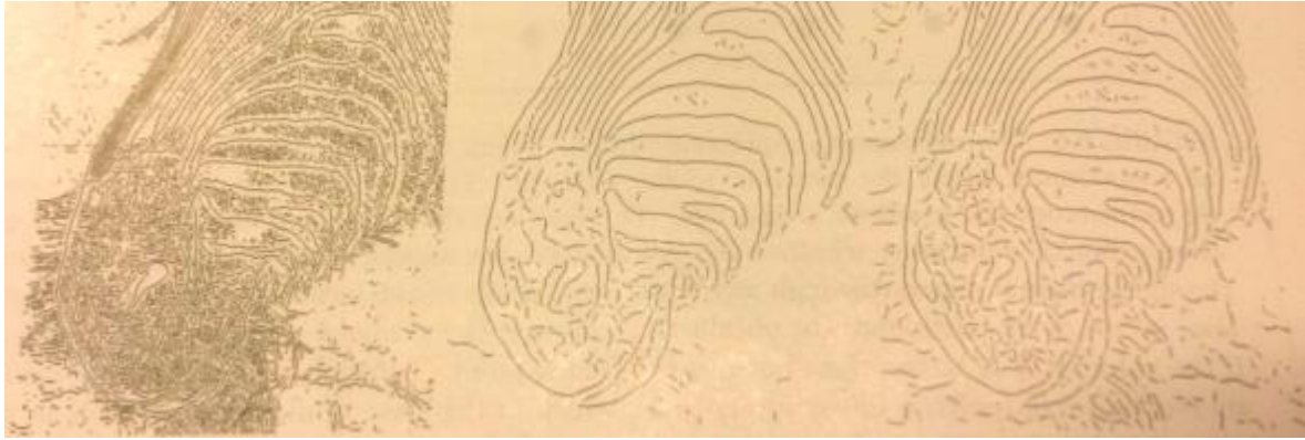
Figure 2-3. Left: Gaussian smoothing scale of \sigma = 1 pixel with high threshold for the gradient magnitude edge point determination. Center: \sigma = 4 pixels with high threshold for the gradient magnitude edge point determination. Right: Low threshold testing and of \sigma = 4 pixels for the gradient magnitude edge point detection (Forsynth and Ponce, 2012).
