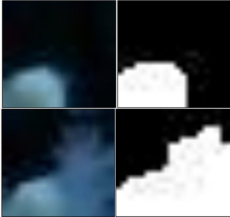
Figure 4-2. The two top images are showing Coral 2, Polyp 4 as seen in Figure 4-7. The cut out image that's being analyzed has a dimension of 20 x 19 pixels. Top left image is showing the image inside red rectangle before threshold. Top right is the same image after threshold. Bottom left is also showing Coral 2 polyp 4 and its thresholded image. The images are showing the results from the software analysis performed on the exact images seen in Figure 4-1.
