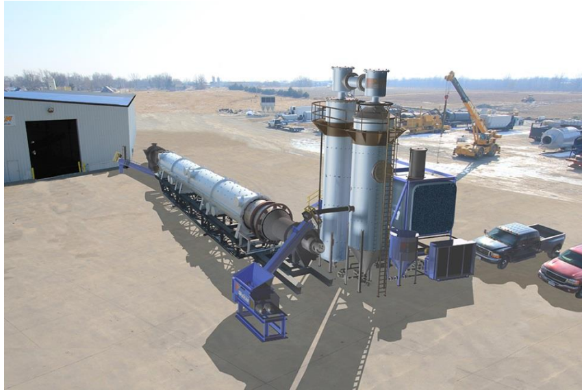
Figure 2.18: Onshore rotary kiln thermal desorption unit for treatment of drill cuttings [25]
