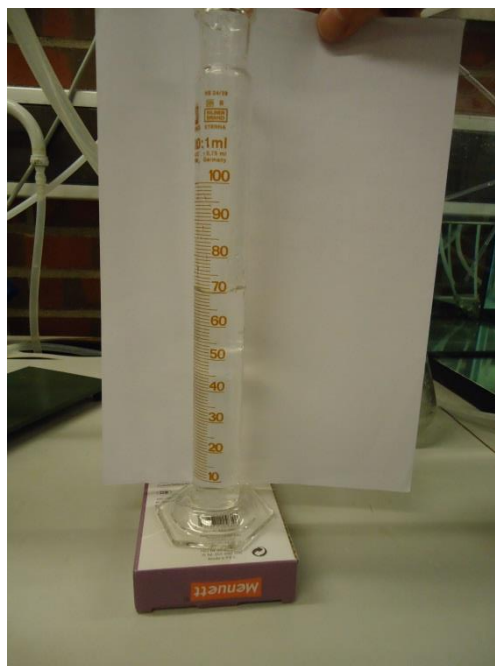
Figure 4.20: Photo of graduated cylinder used to capture condensed vapors
