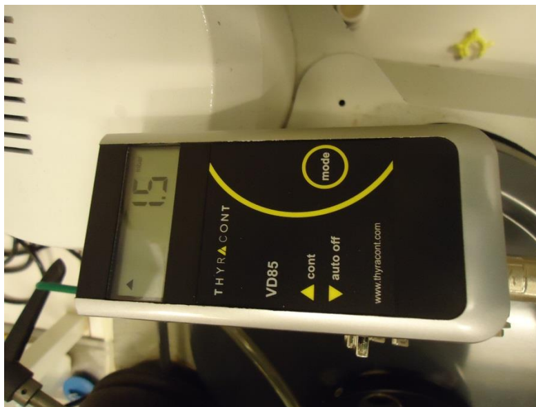
Figure 4.5: Photo of pressure gauge (Thyracont Model VD85) associated with the high powered two stage vacuum pump
