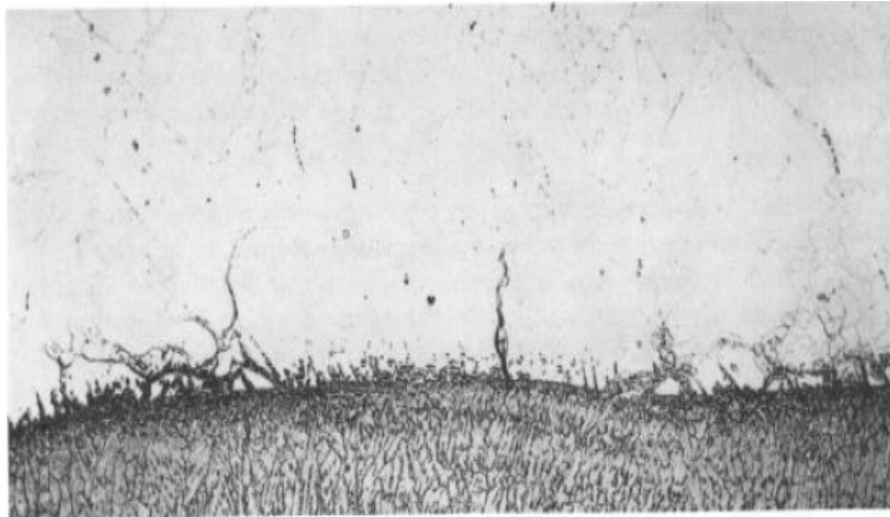
Figure 2-9: Liquation cracks in the grain boundaries in the HAZ of gas-tungsten-arc welded Inconel 718 [4].
