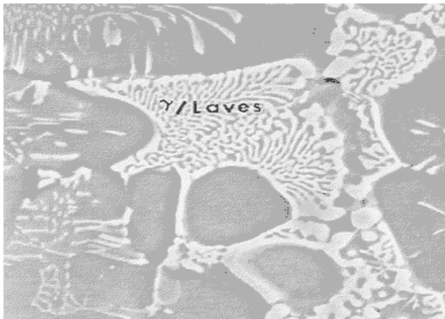
Figure 2-4: Laves phase in a eutectic formation with \gamma -austenite after solidification [13].
