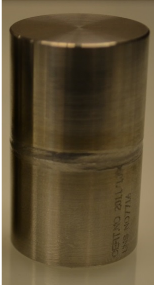
Figure 3-4: Corrosion specimen after electron beam welding.
