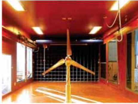
Figure 1: The model wind turbine in the wind tunnel, NTNU.
