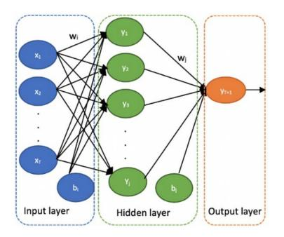
Figure 1: Architecture of applied Artificial Neural Network (ANN)
