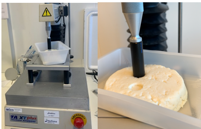
Figure 3.5 TA.XT Plus Texture Analyser (Stable Micro Systems Ltd., Godalming, UK) with a cylinder probe (Delrin cylinder P/0.5R, Stable Micro Systems Ltd., Godalming, UK) attached.
