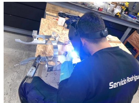
Figure 4.21 – TIG welding aluminium brackets and hoops to mid-plate
