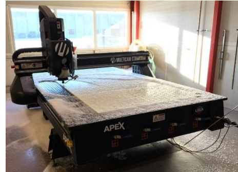
Figure 4.23 – Apex Multicam CNC router, cutting side plates
