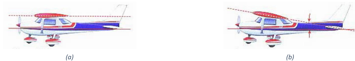
Figure 5.12 – Effect of angle of attack on a wing. (a) No angle of attack, and (b) Pressure difference created by angle of attack (Marine, 2004).
