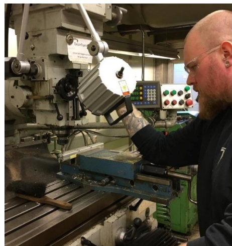
Figure 4.18 – Milling parts of the ROV-frame at the University of Stavanger
