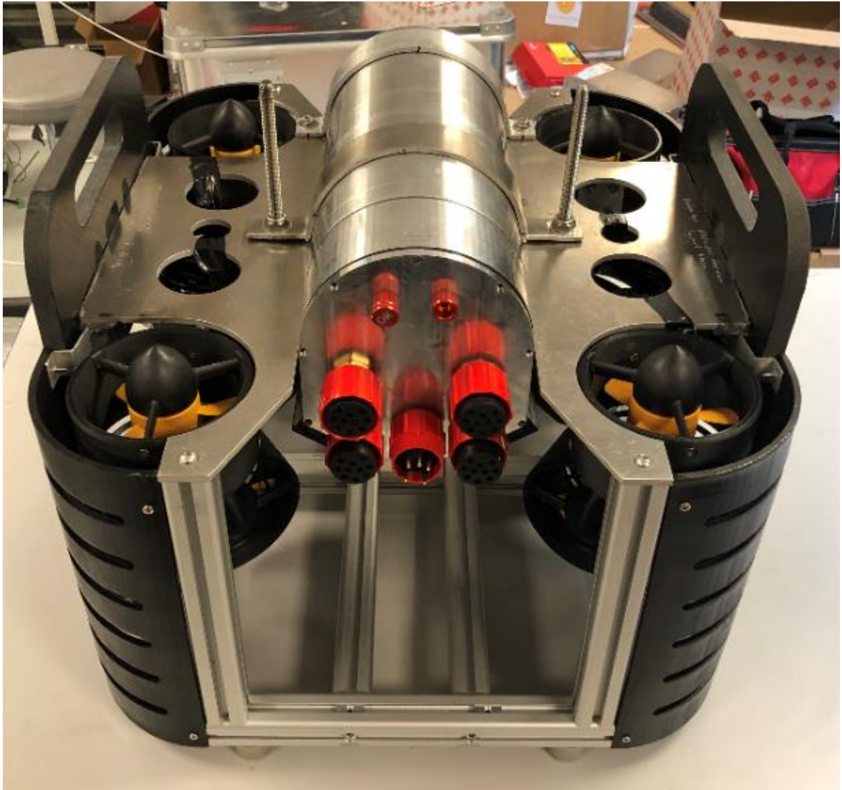
Figure A.3 – Rear view of Hymir, showcasing its electronic container and four vertical thrusters
