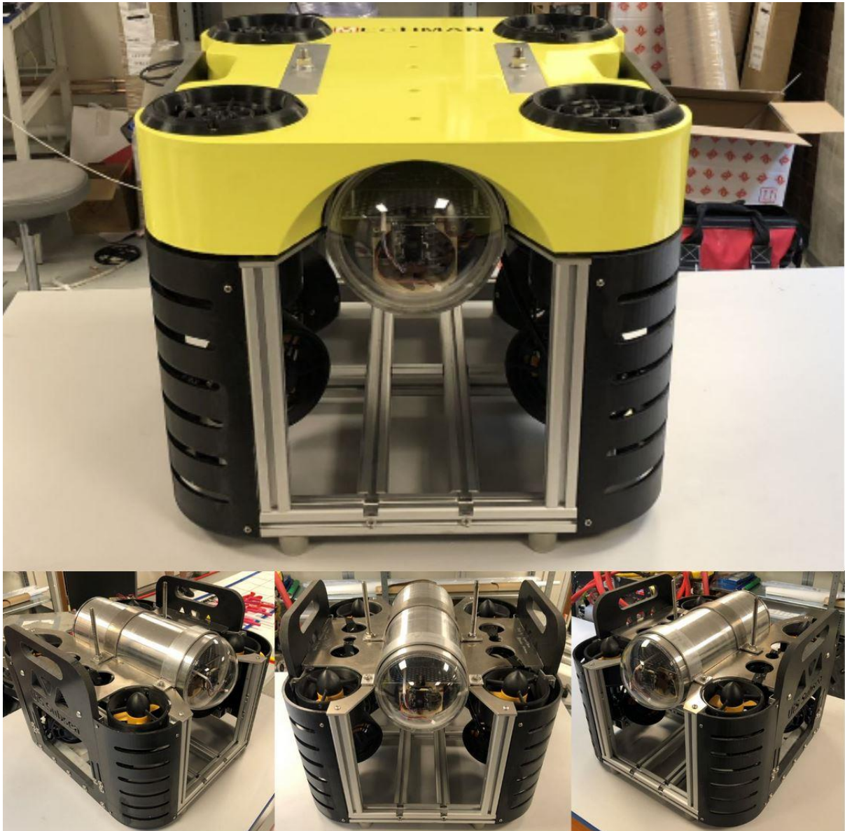
Figure A.1 – Hymir showcasing its (yellow) buoyancy foam at the top, and the electronic container in the centre of the frame
