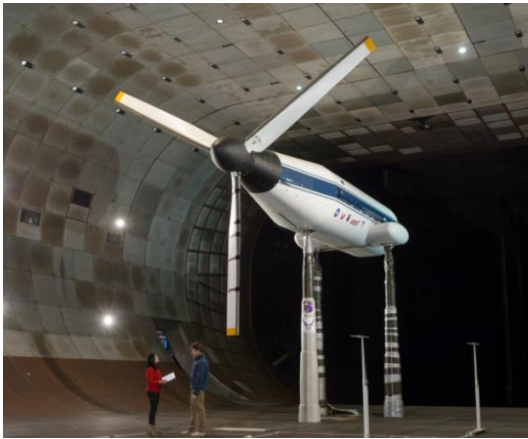
Figure 4.4 Inside the world largest wind tunnel at NASA Ames Research Center in California. Photo showing test rig for rotor blade (Photo courtesy of NASA Ames Research Center).
