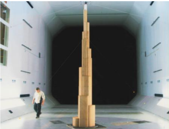
Figure 4.3: Wind tunnel testing of a model of Burj Khalifa (Photo courtesy of RWDI Consulting Engineers).
