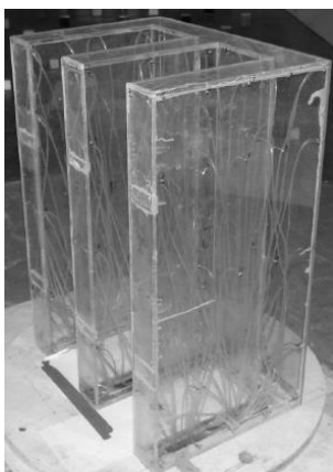
Figure 7.1: Model of E-shaped building used in wind tunnel testing, scale 1:300 (left). Isometric drawing of E-shaped building (right) [67].
