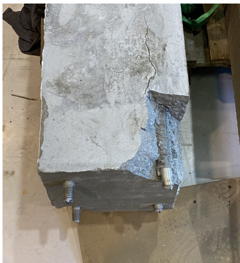
Figure 4.6: Threaded section after surpassing maximum design resistance
