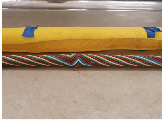
Figure 2.3: Z-kinks discovered by IKM upon inspection of tether. Image provided by IKM.
