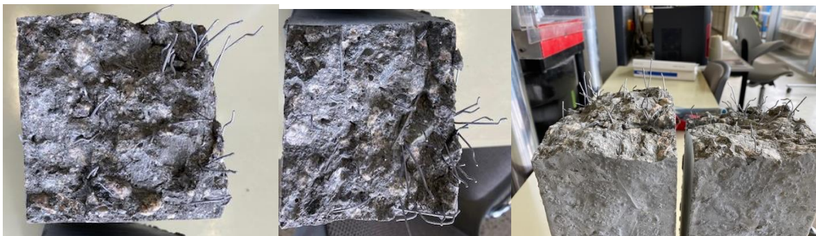
Figure 3-21: Cracked cross section of SFRC specimen
