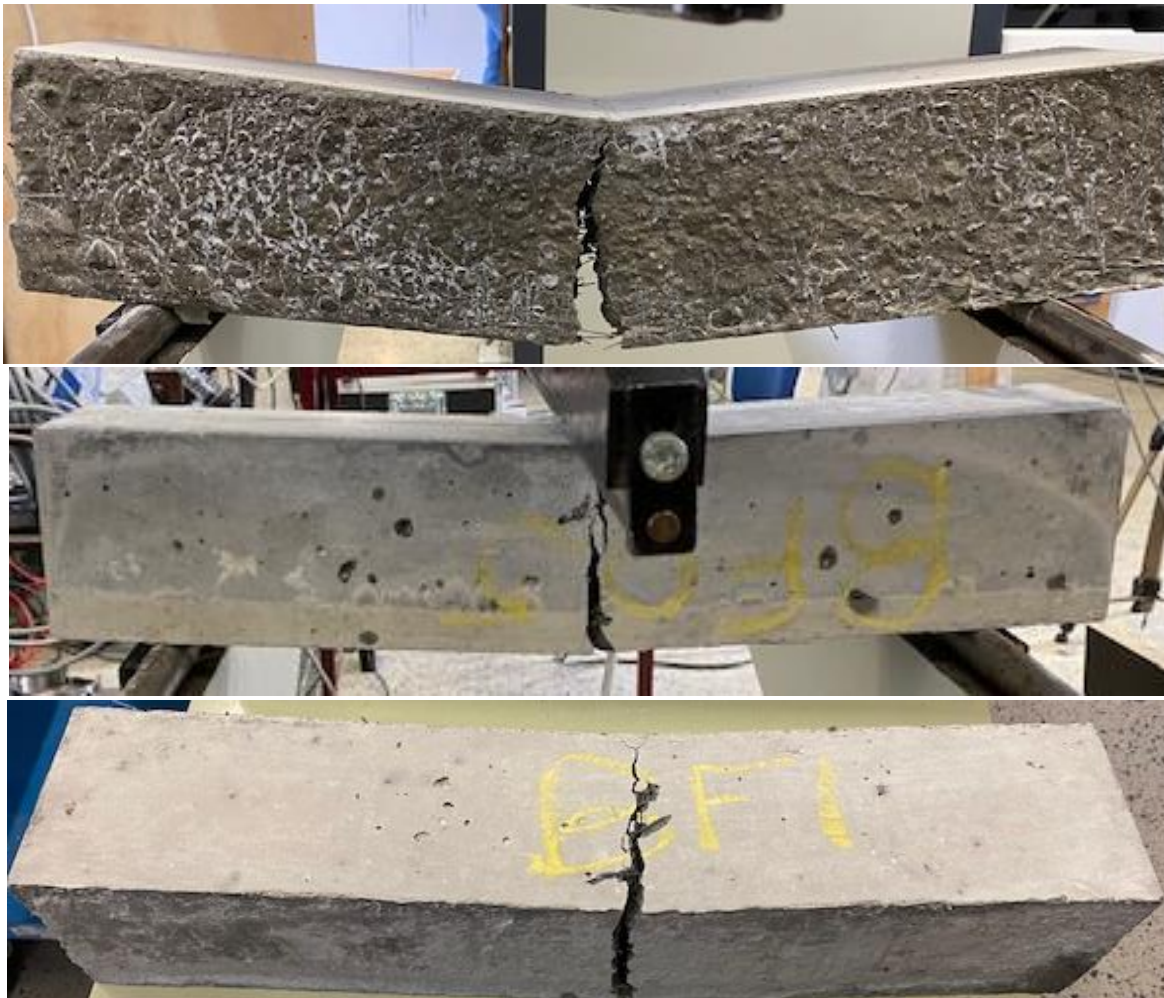
Figure 3-22: Failure mode of a) day 1 0.5% BFRC b) day 28 0.5% BFRC c) day 28 1% BFRC
