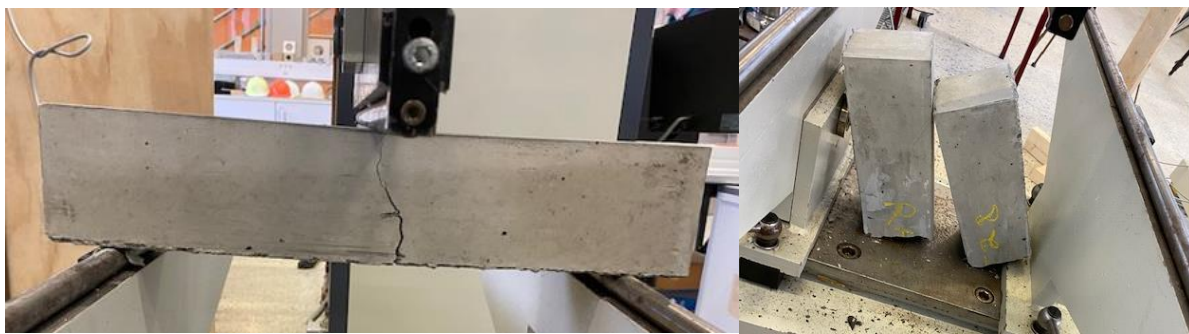
Figure 3-18: Flexural failure of plain concrete a) day 1 specimen b) day 28 specimen
