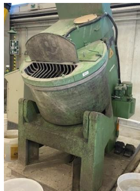
Figure 3-3: The concrete mixer used
