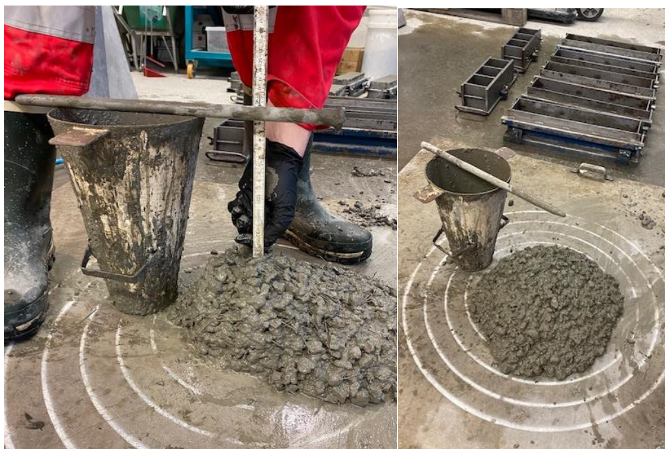
Figure 3-4: Technique used to measure the slump
