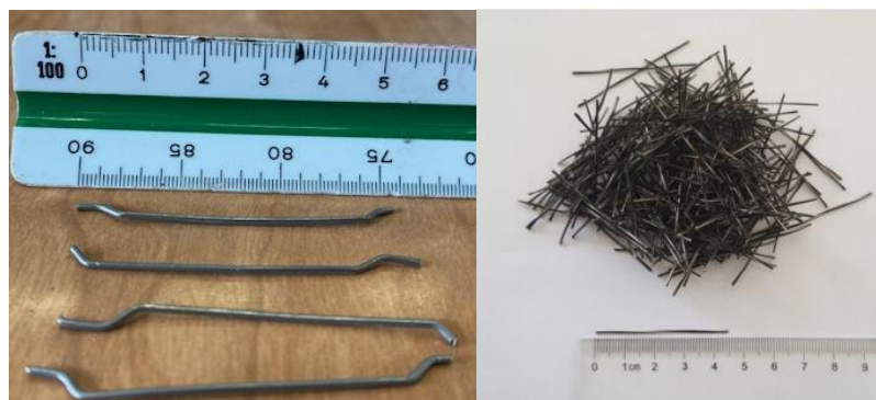
Figure 3-1: a) The steel fibers used, b) The basalt fibers used
