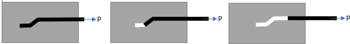
Figure 3-19: How failure by pullout occurs
