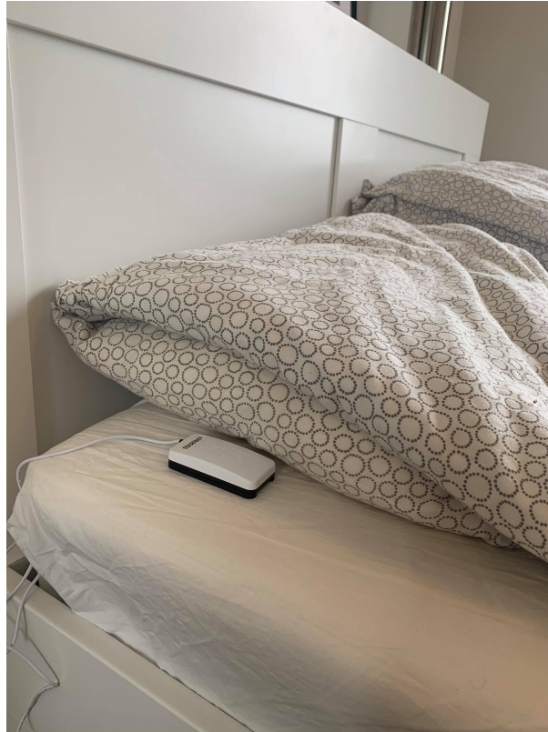
Figure 3.2: Sensor that is used to measure the patients vitals.
