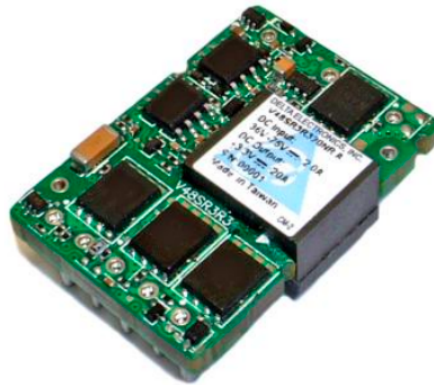
Figur 2.13: Delphi Series V48SR, 1/16 th Brick 65W DC/DC [30].
