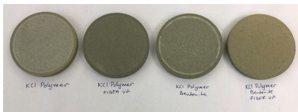
Figure 9. Discs from tests 12–15 after breaker application and drying.
