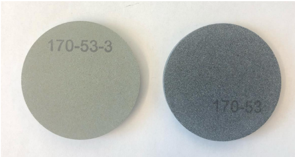
Figure 1 - OFITE ceramic discs. 20\mu\text{m} disc to the left and 50\mu\text{m} disc to the right.
