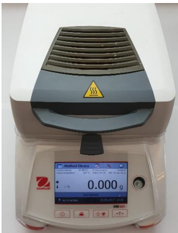
Figure 6 - OHAUS MB120 moisture analyzer, used for removing moisture and determining disc mass.
