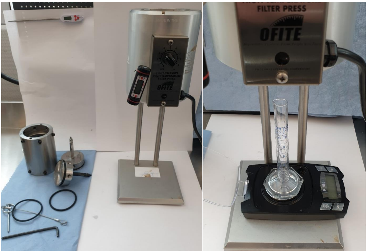
Figure 4 - To the left is the OFITE HTHP Filter Press in parts, used for conducting fluid loss tests. To the right are the scale and a measuring cylinder used for recording the fluid loss.
