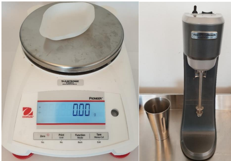
Figure 2 - To the left is the scale, Ohaus ax1502, used for measuring all components. To the right is the Hamilton beach mixer.
