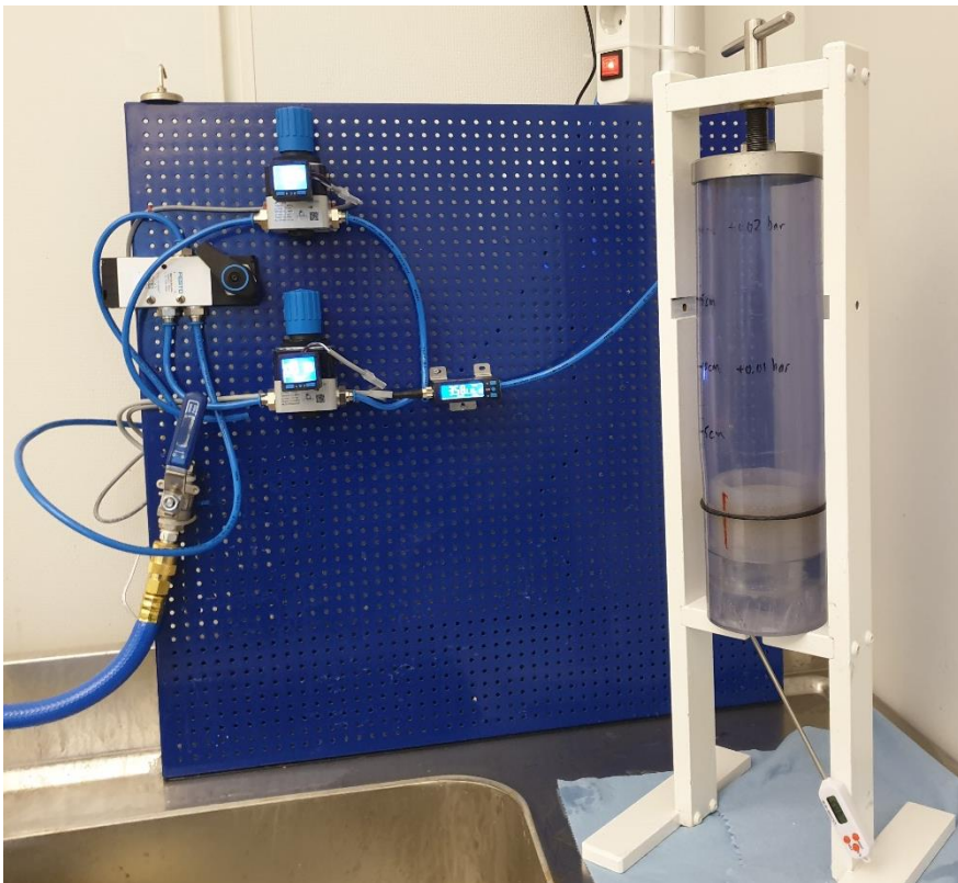
Figure 5 - Custom setup for filter cake removal and permeability measurements.
